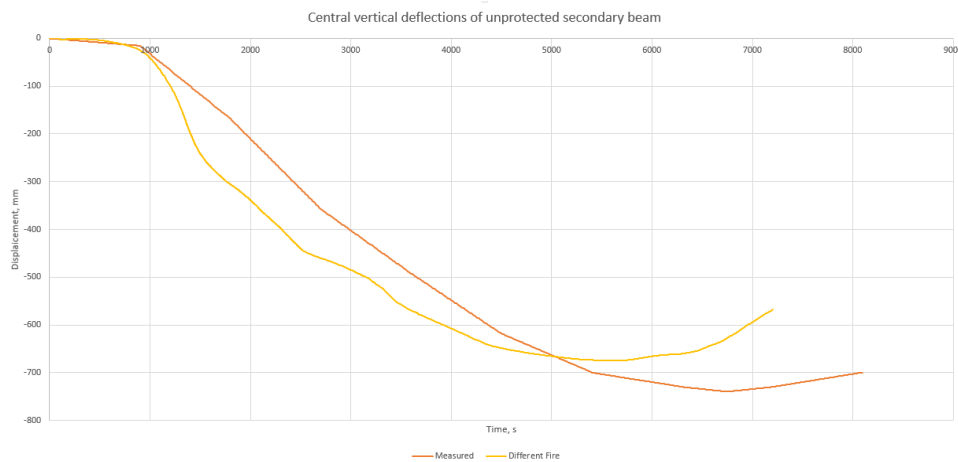
Fig. 5.3.1. Comparison between measured and computed vertical deflection at the middle of the unprotected beam
