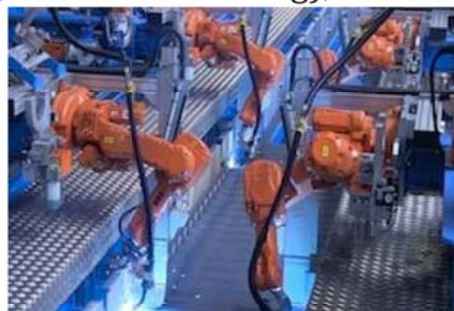
Figure 11. Zeman fully-automated SIN-beam production.
