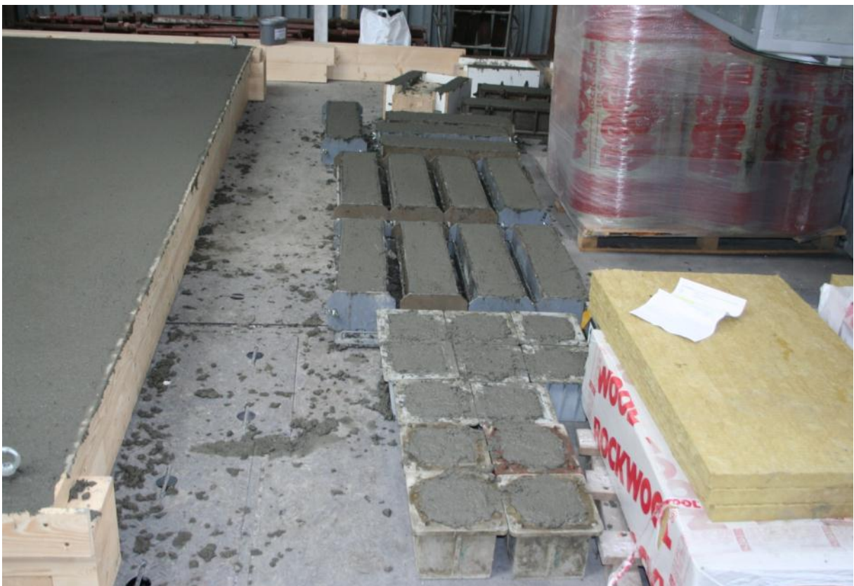
Concreting of the cubes, scantlings and specimen for push-out tests
