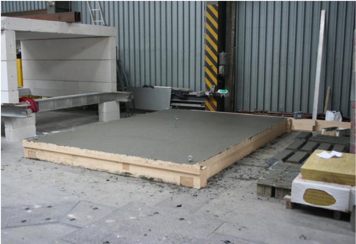
Concreting of the cubes, scantlings and specimen for push-out tests
