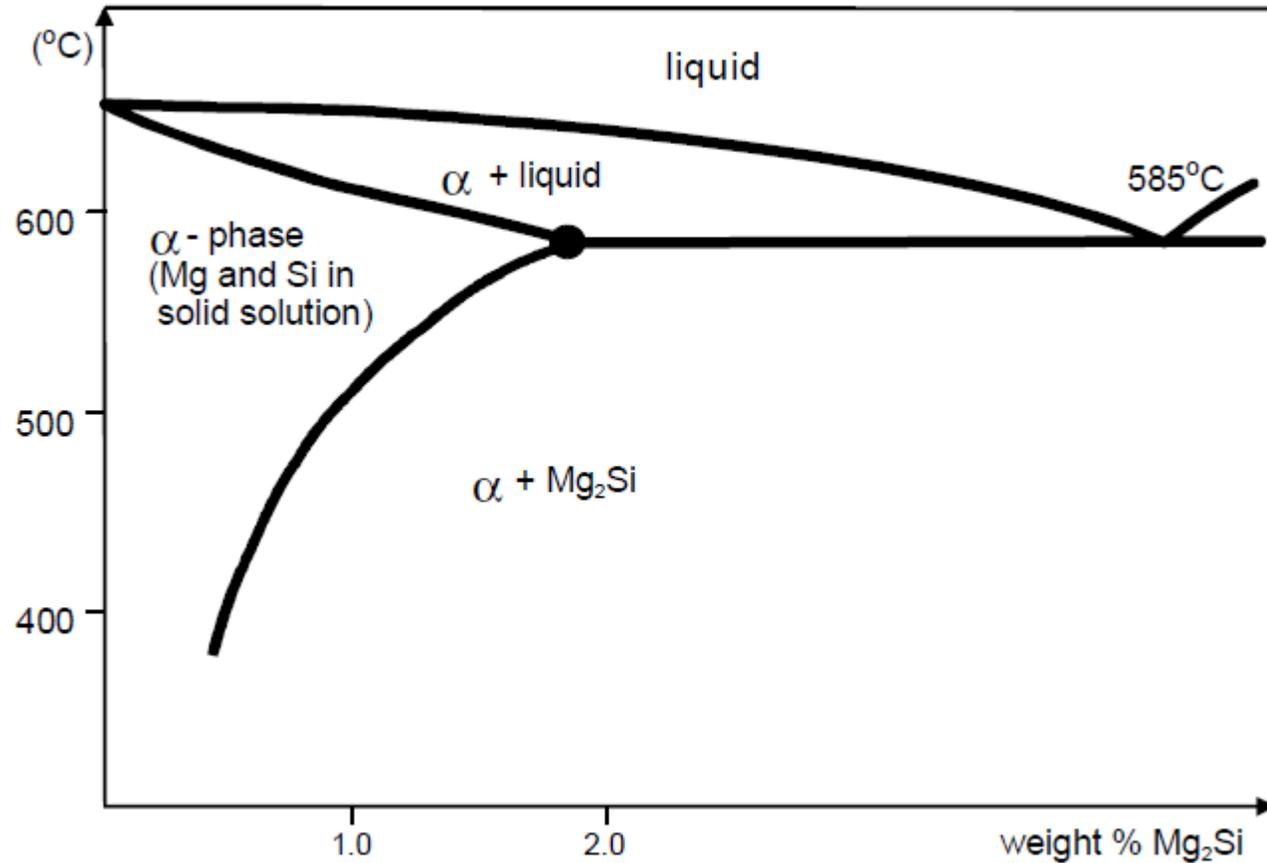
Example of phase diagram for Mg<sub>2</sub>Si in aluminium
