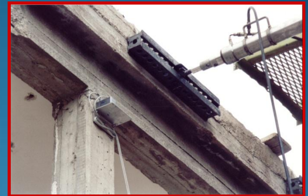
Close-up views of the reacting structure with the load jacks
