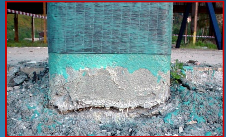
Close-up views of plastic hinges at the column bases
