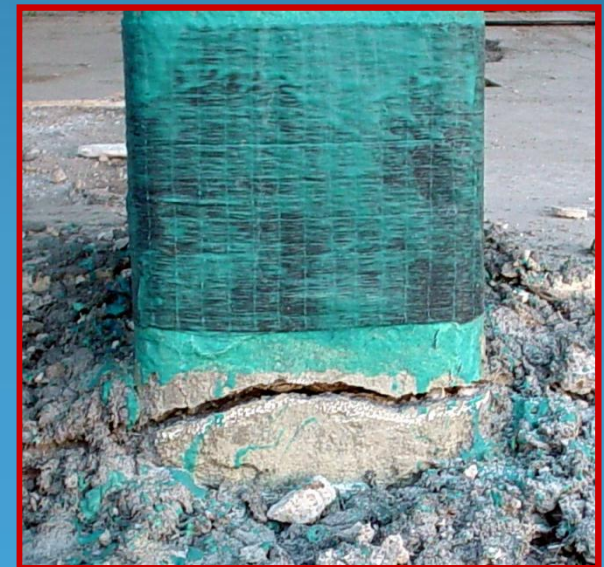
Close-up views of plastic hinges at the column bases
