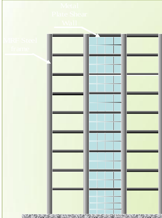
MRF+Shear Panels (Dual Structural System)
