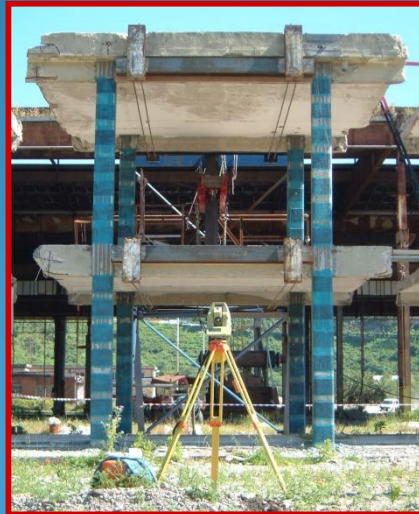
Displacement measuring devices
