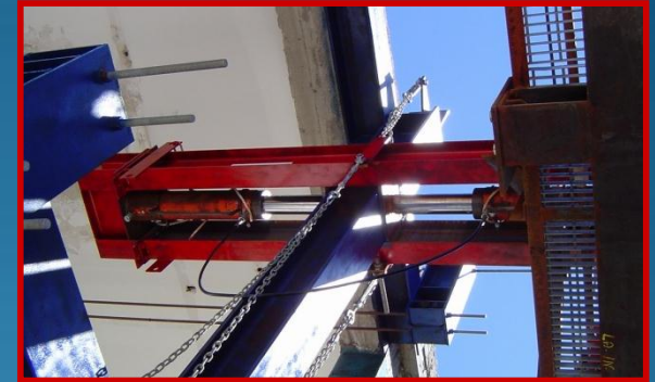
Close-up views of the reacting structure with the load jacks
