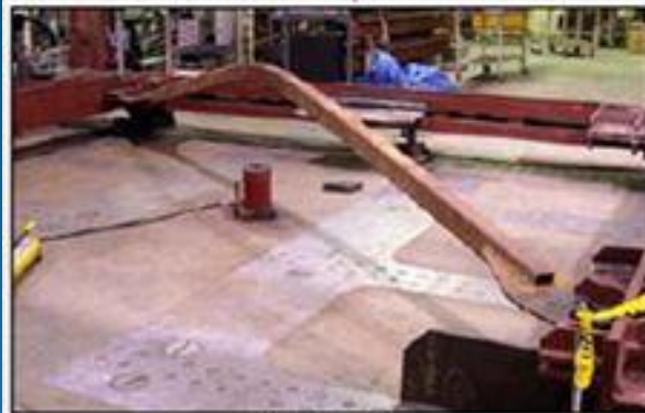
- Buckled out - Poor nonlinear behaviour
