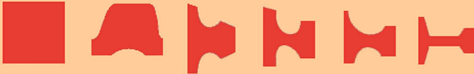
D: Progressive shaping of a bloom into a rail.
