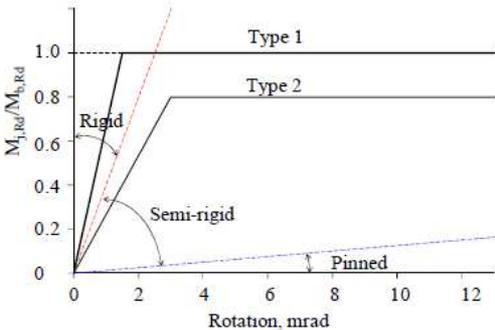
Figure 16 Moment-rotation curve for connections
