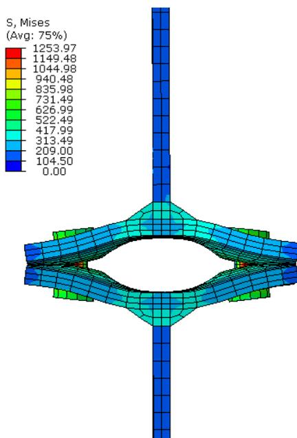
Figure 45 Stresses before failure
