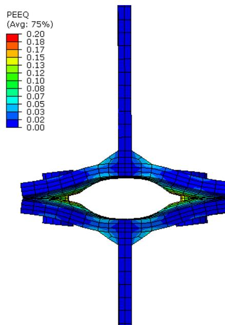
Figure 44 PEEQ before failure
