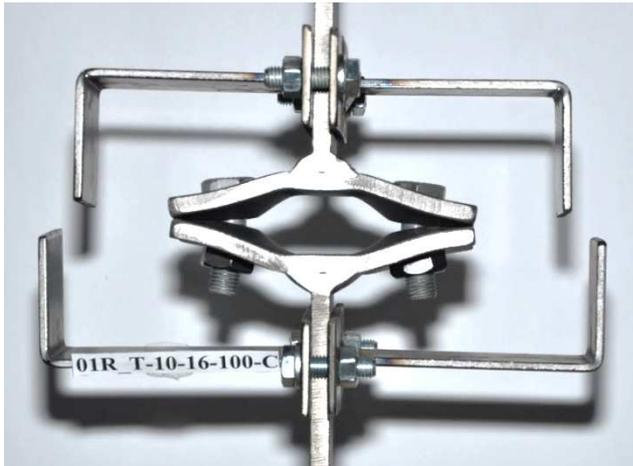
Figure 43 Photo of T-stub just before failure
