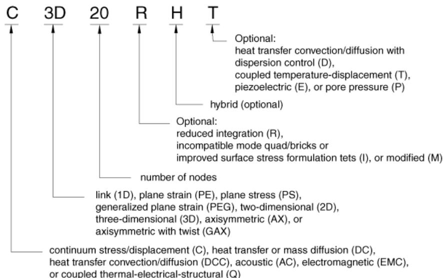
Figure 27 Name convention of solid elements in Abaqus
