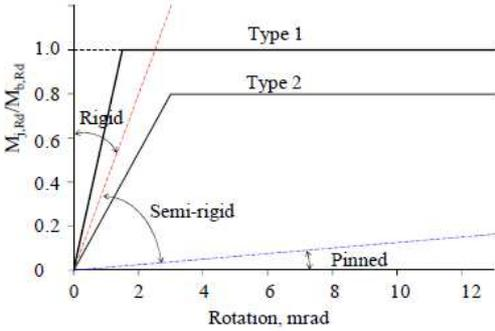
Figure 16 Moment-rotation curve for connections
