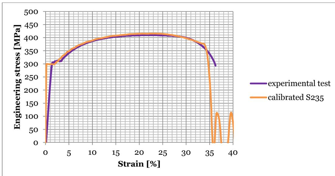
Figure 40 Coupon curve
