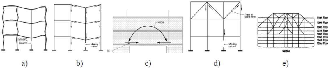
Figure 10 Supplementary load transfer routes (Marginean, 2013)
