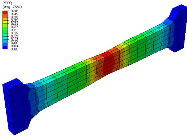
Figure 38 PEEQ before failure
