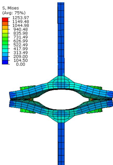
Figure 45 Stresses before failure
