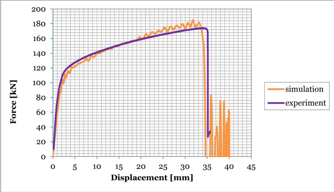
Figure 46 Force displacement curve of T-stub
