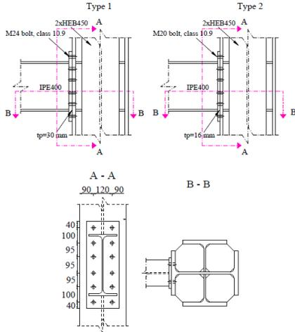
Figure 15 Connection details of beam-to-column
