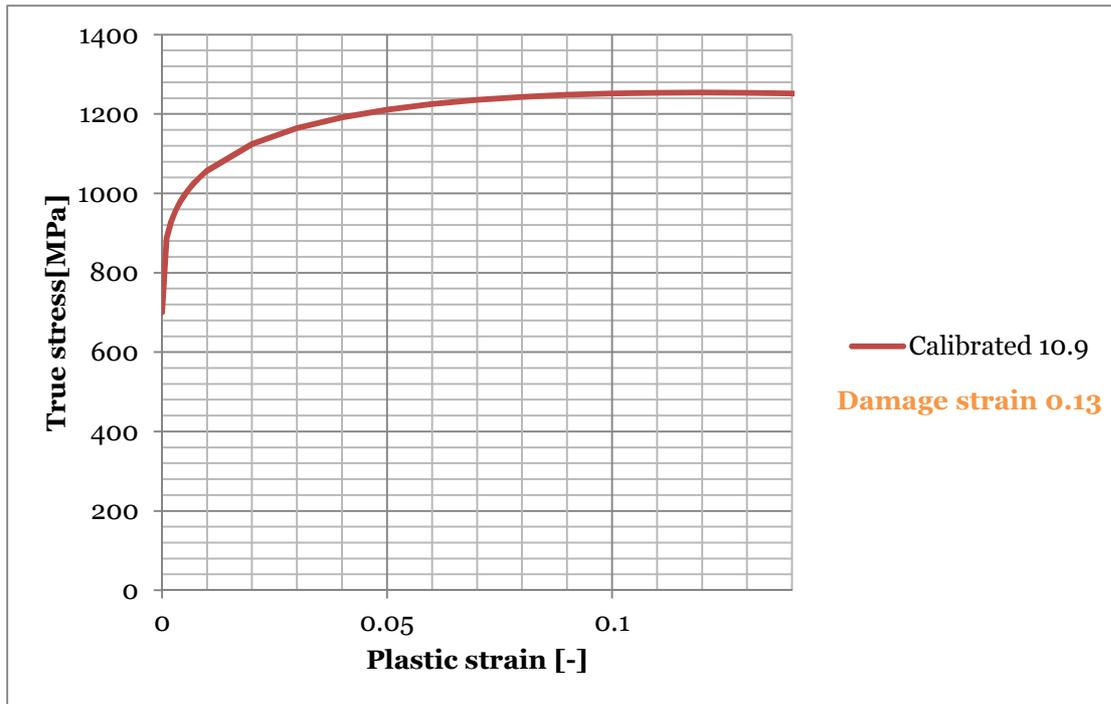
Figure 31 Bolt 10.9 plastic curve
