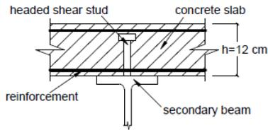
Figure 13 Cross-section of composite secondary beam
