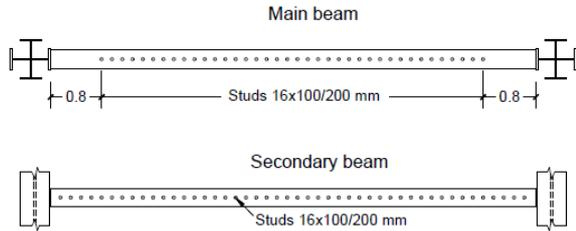
Figure 14 Spacing of connectors for main and secondary beams
