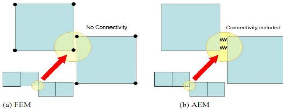
Figure 17 Partial element connectivity (Source: ELS Theoretical Manual)
