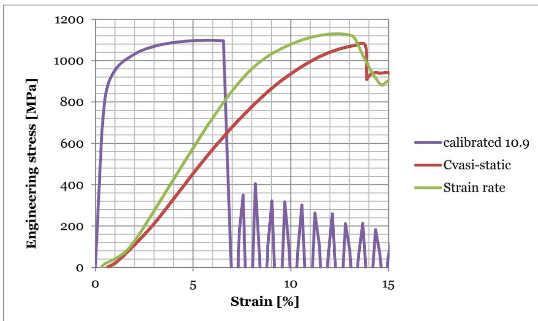
Figure 42 Bolt curve
