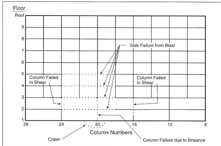
Figure 3 Damage of Murrah building directly after explosion
