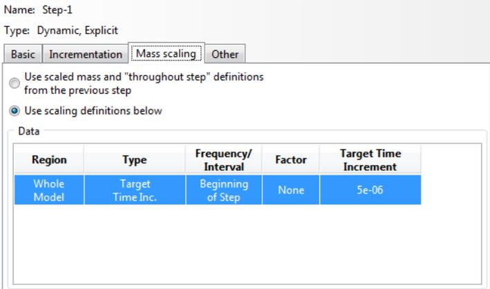
Figure 34 Mass scaling of the model
