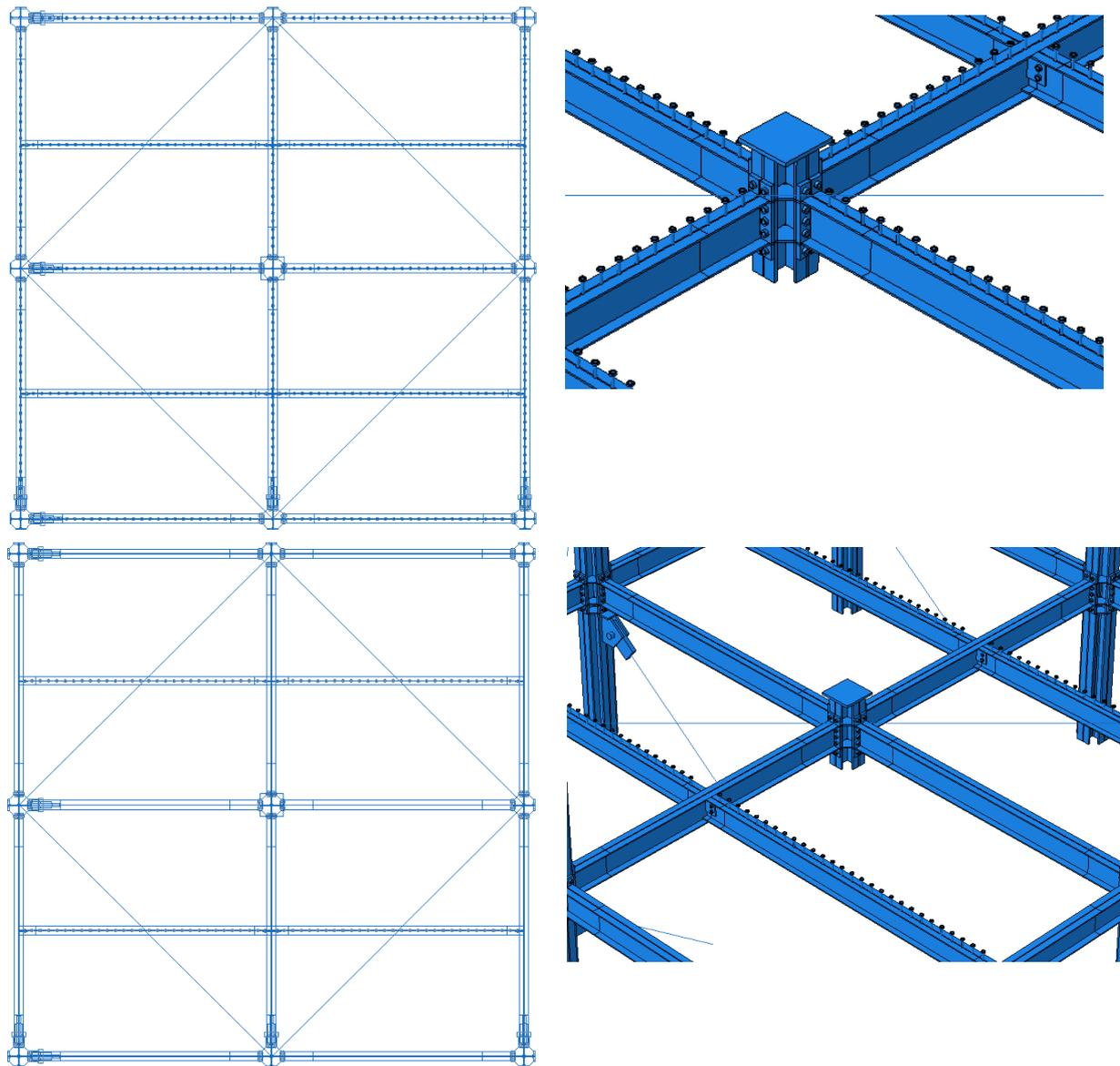
Figure 4.74 Spacing of the shear connectors for the two scenarios
