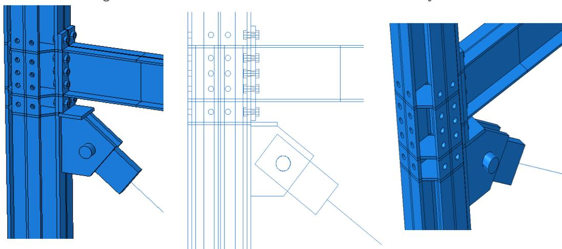
Figure 4.38 Bracing system connection detail in Abaqus
