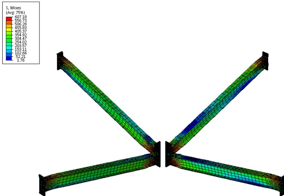
Figure 4.54 Stresses in the beams at a displacement of 800 mm, load of 1086 kN
