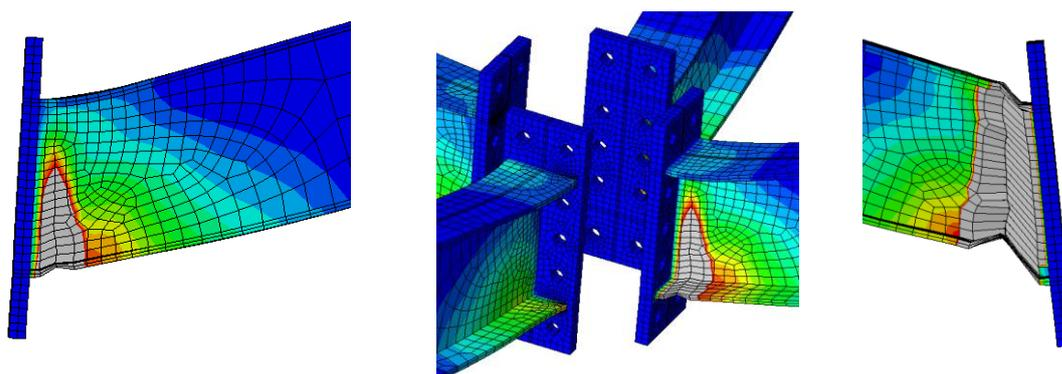
Figure 4.46 Failure of the structure at a displacement of 692 mm, load of 852 kN
