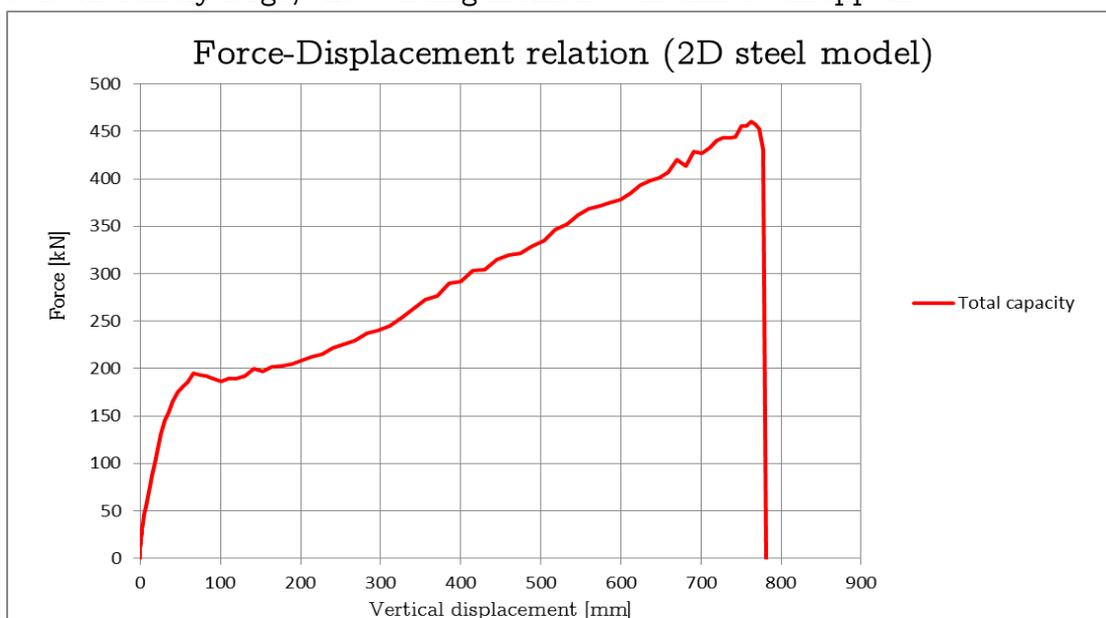
Figure 4.81 Force-Displacement relation for the total applied loading (2D steel model)
