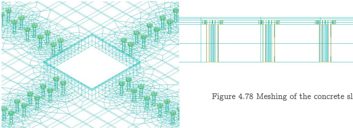
Figure 4.78 Meshing of the concrete slab
