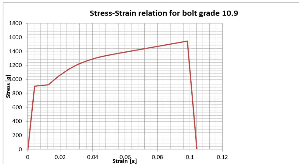
Figure 4.12 Stress-Strain relation of bolt grade 10.9
