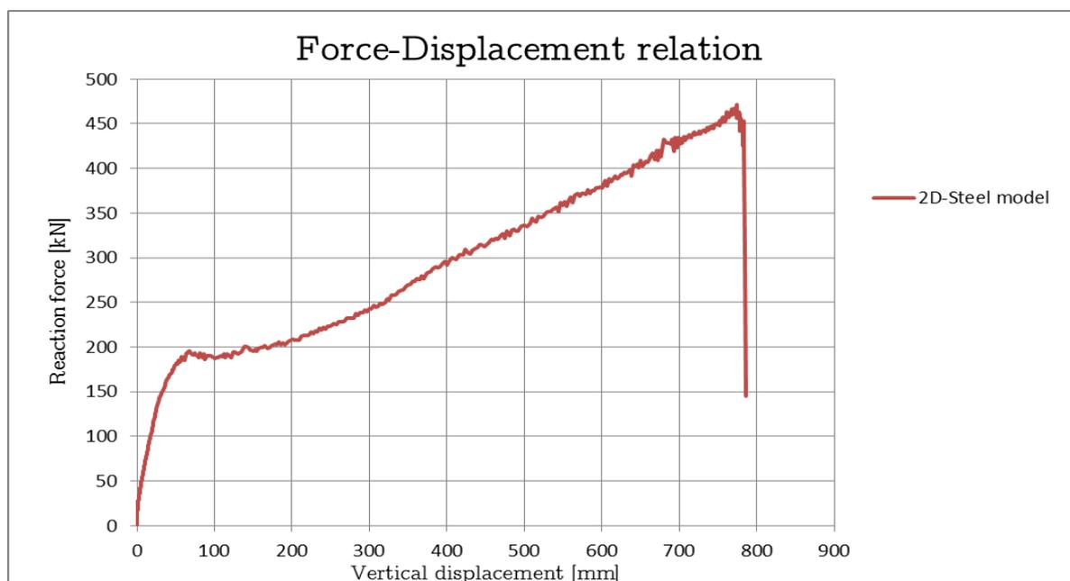
Figure 4.32 Force-Displacement curve for the 2D-model
