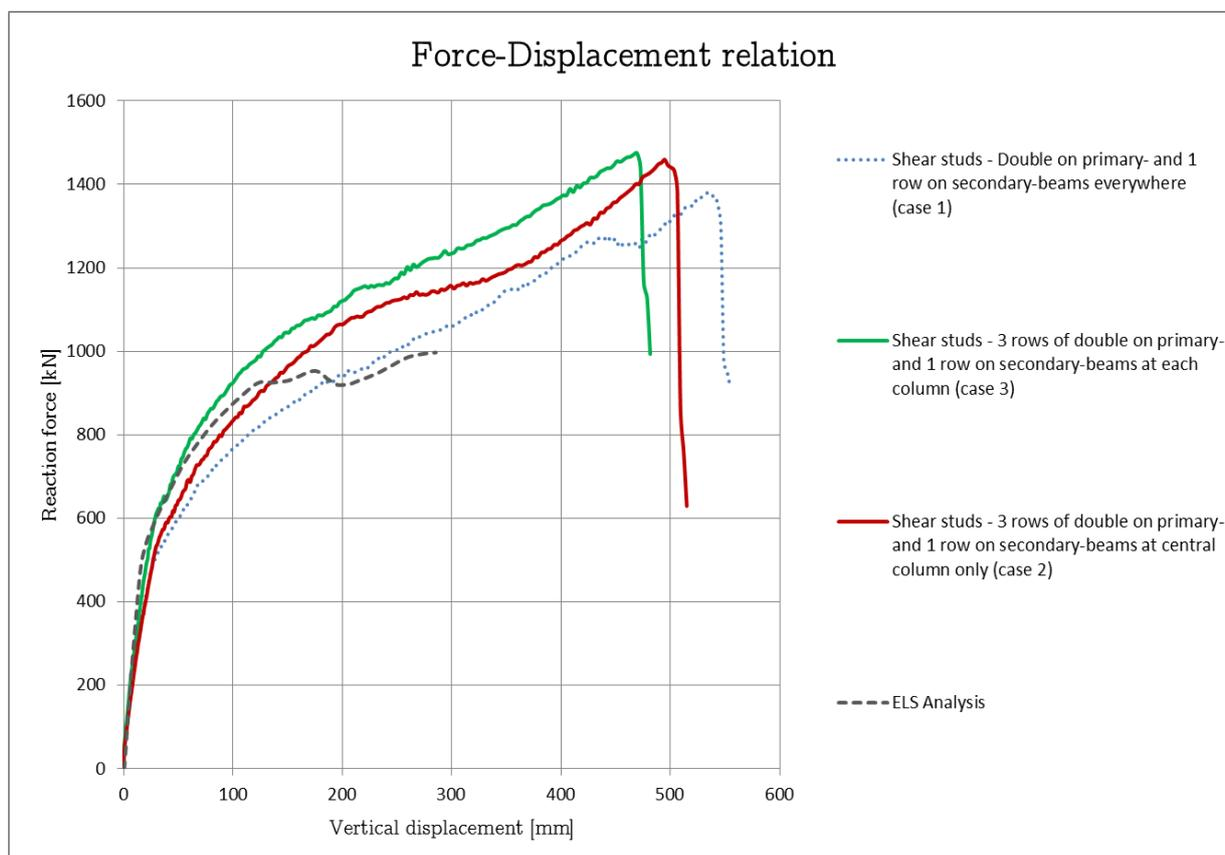
Figure 5.3 Force-Displacement relation for case 1, case 2, case 3 (shear studs) and ELS Analysis
