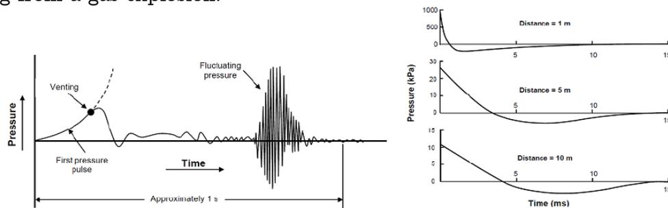
Figure 1.7 Typical time history of the pressure resulting from a gas explosion (left) and from detonation of explosives (right) (Margeinean et al, 2013)
