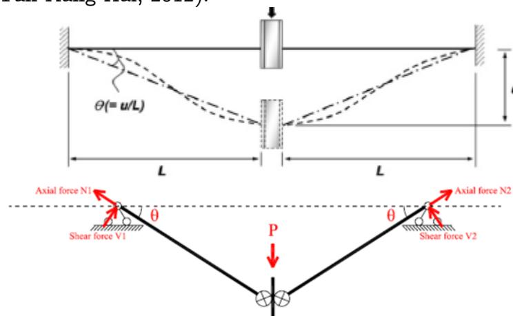
Figure 4.84 Representation of the catenary action mechanism (Lee et al, 2009)
