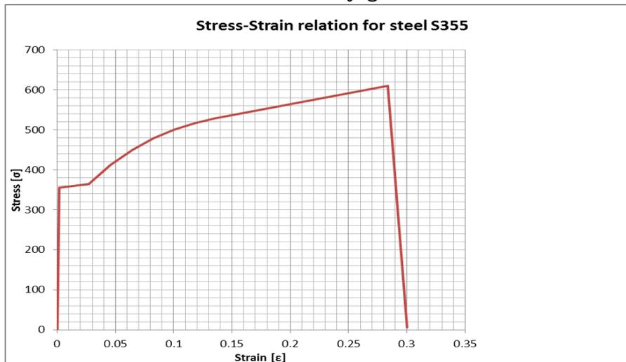
Figure 4.6 Stress-Strain relation of steel S355
