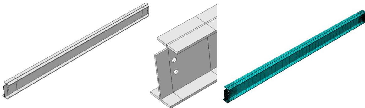
Figure 4.58 Secondary-beam modeling
