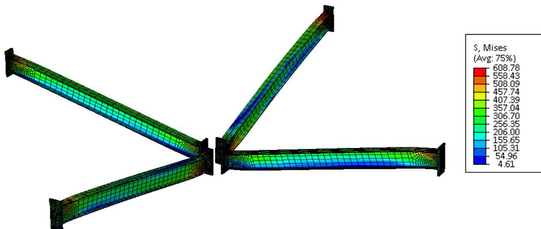
Figure 4.45 Stresses in the beams at a displacement of 692 mm, load of 852 kN
