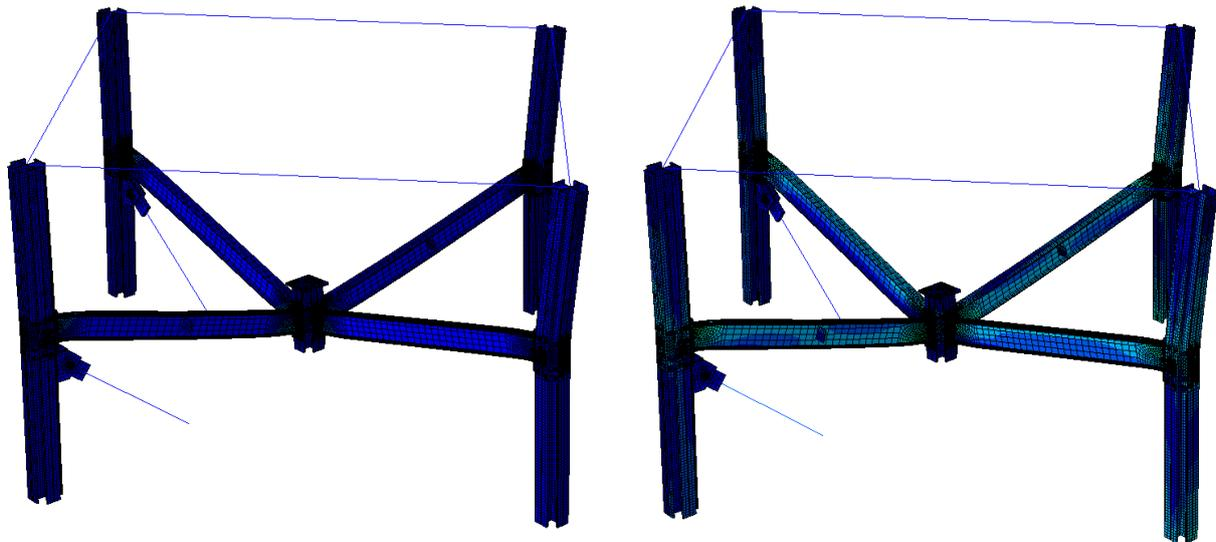
Figure 4.41 Deformed shape of the structure
