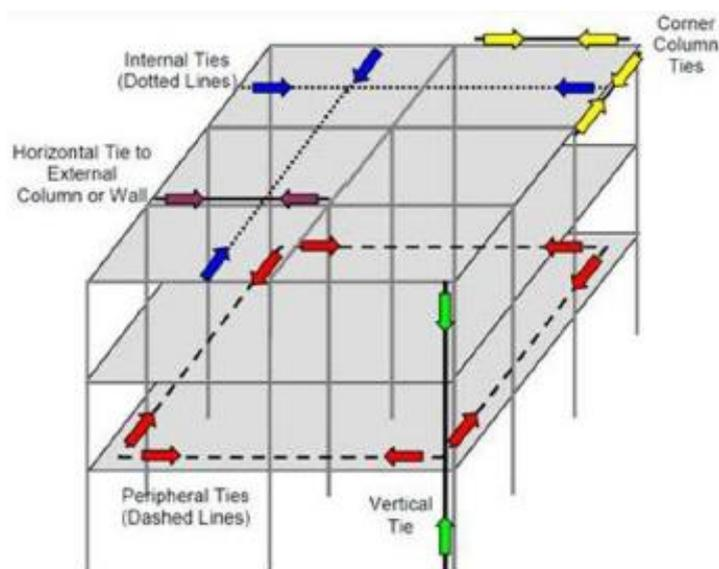
Figure 1.8 Different types of ties incorporated to provide structural integrity (DOD, 2005)
