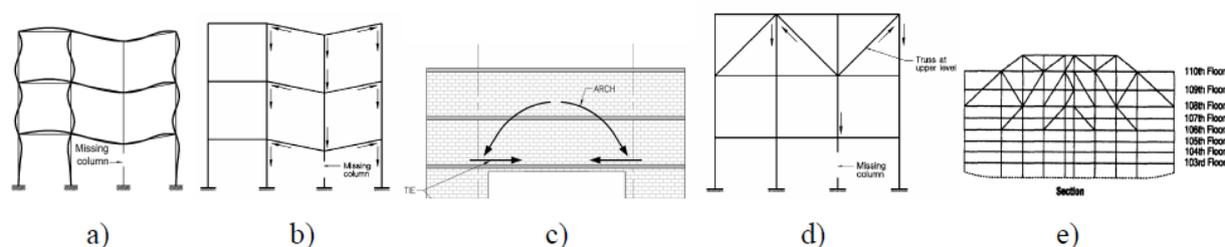
Figure 1.13 Supplementary load transfer routes: a) Vierendeel action; b) Catenary action; c) Arch effect; d) Suspension effect; e) Hat trusses on top of WTC (suspension effect) (Marginean, 2013)
