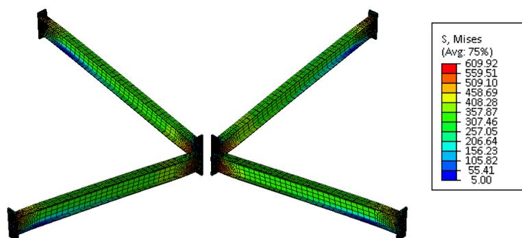
Figure 4.72 Stresses in the beams at a displacement of 542 mm, load of 1324
