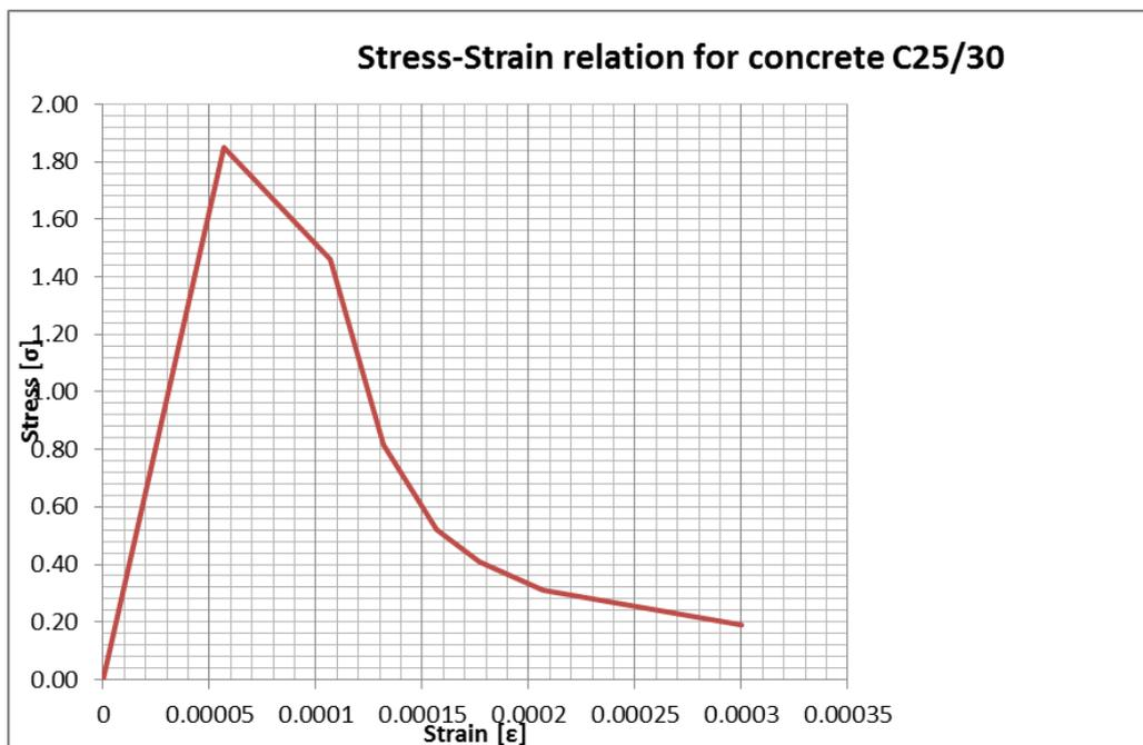
Figure 4.9 Stress-Strain relation of concrete C25/30 (tensile behavior)
