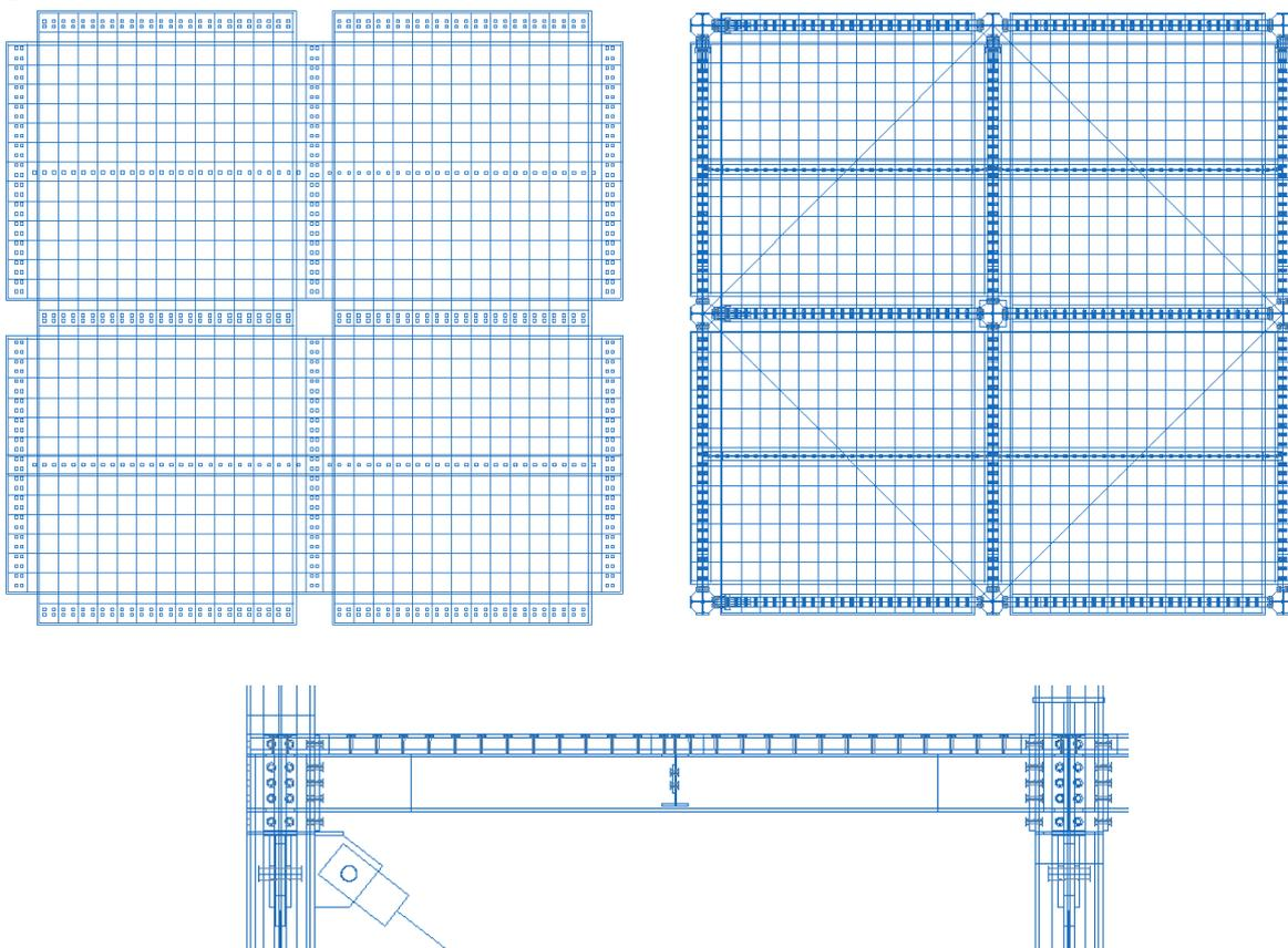
Figure 4.64 Spacing of the reinforcement within the concrete slab in Abaqus
