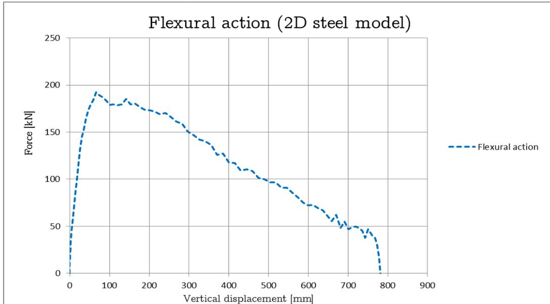
Figure 4.82 Contribution of the flexural action for the total applied loading (2D steel model)
