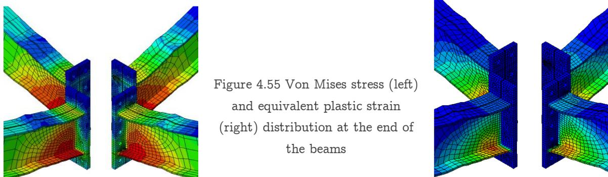
Figure 4.55 Von Mises stress (left) and equivalent plastic strain (right) distribution at the end of the beams
