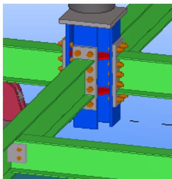
Figure 4.4 Removal of the key element (column)
