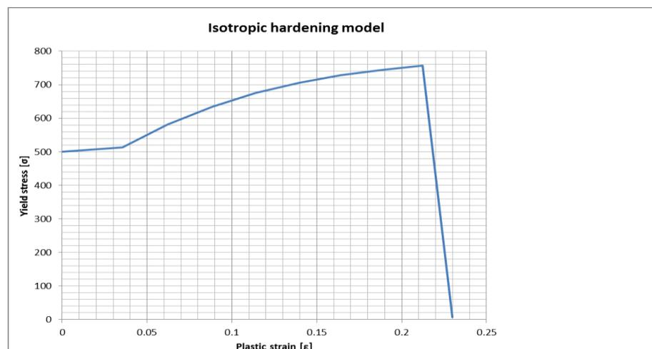
Figure 4.11 Isotropic hardening model data used for defining the nonlinear plastic behavior of steel
