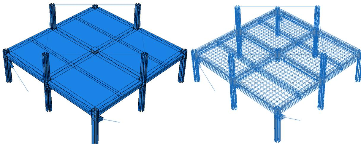
Figure 4.62 Shaded and wireframe view of the 3D composite model
