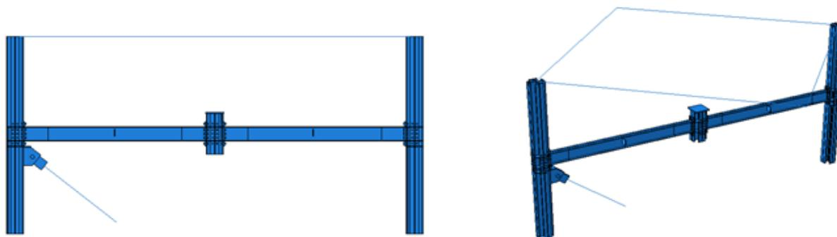
Figure 4.14 Finite element model of the central frame of the sub-assembly
