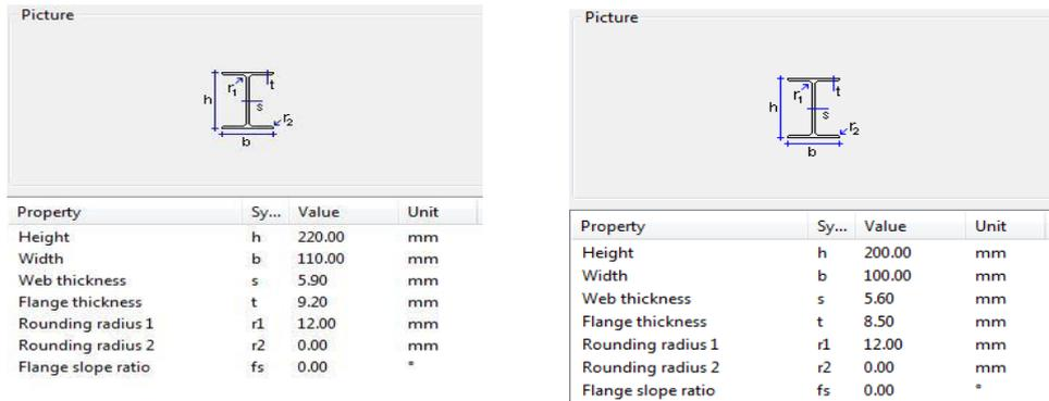
Figure 3.10 Primary beam (left) and secondary beam (right) cross-sectional characteristics
