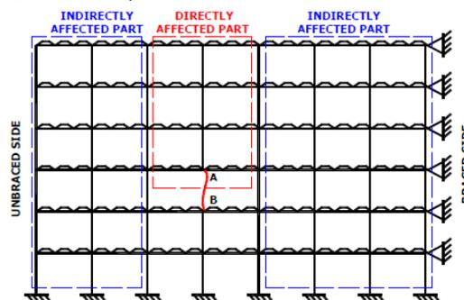
Figure 1.15 Directly and indirectly affected part (Hai, 2009)
