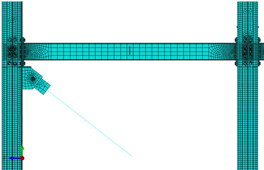
Figure 4.40 Mesh defined for the primary-beam
