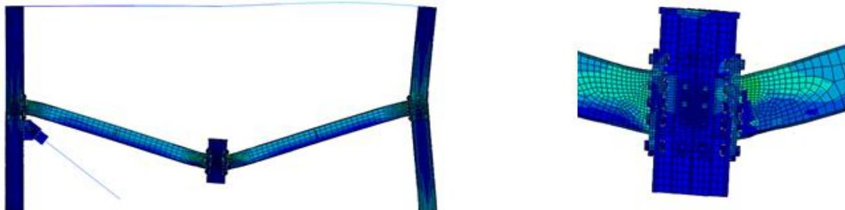
Figure 4.36 Rotation tendency of the loaded column (2D model)
