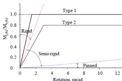
Figure 3.5 Moment-rotation curve for connections (Marginean et al, 2013)
