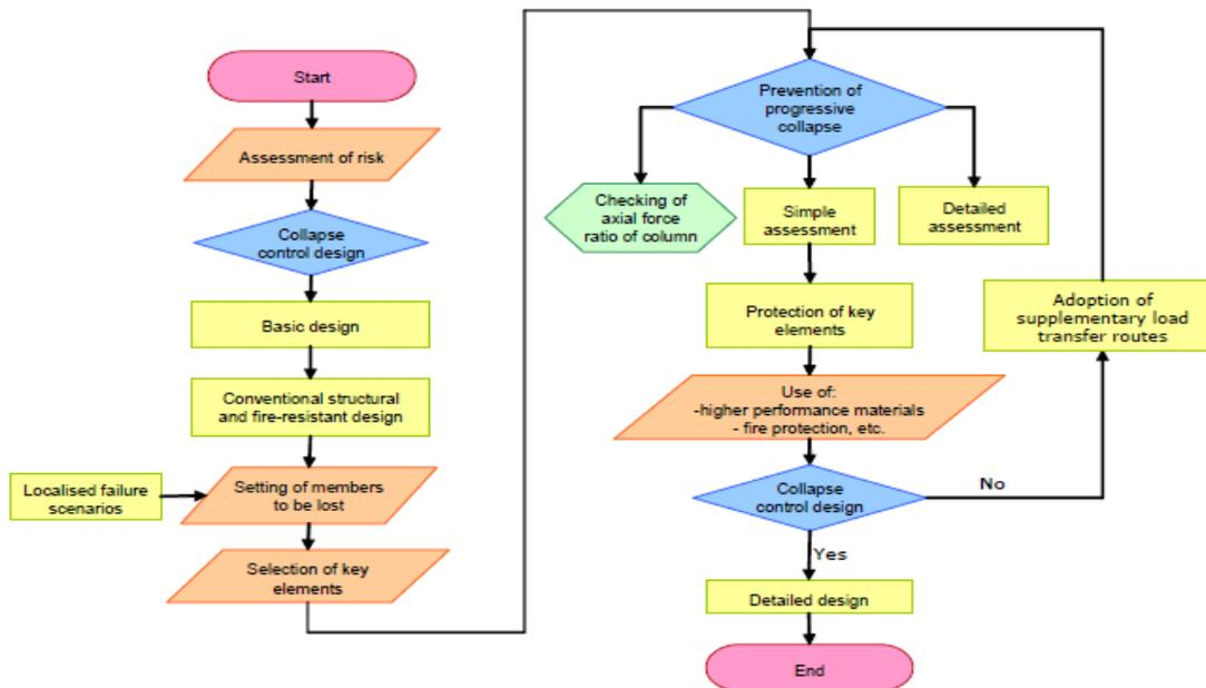
Figure 1.12 Collapse control design flowchart (Marginean et al, 2013)
