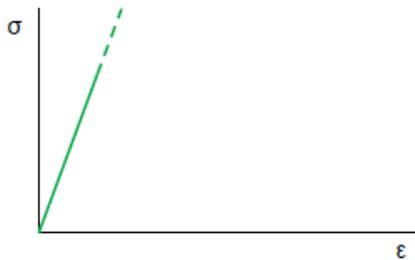
Figure 4.5c Typically linear-elastic material model (Arup)
