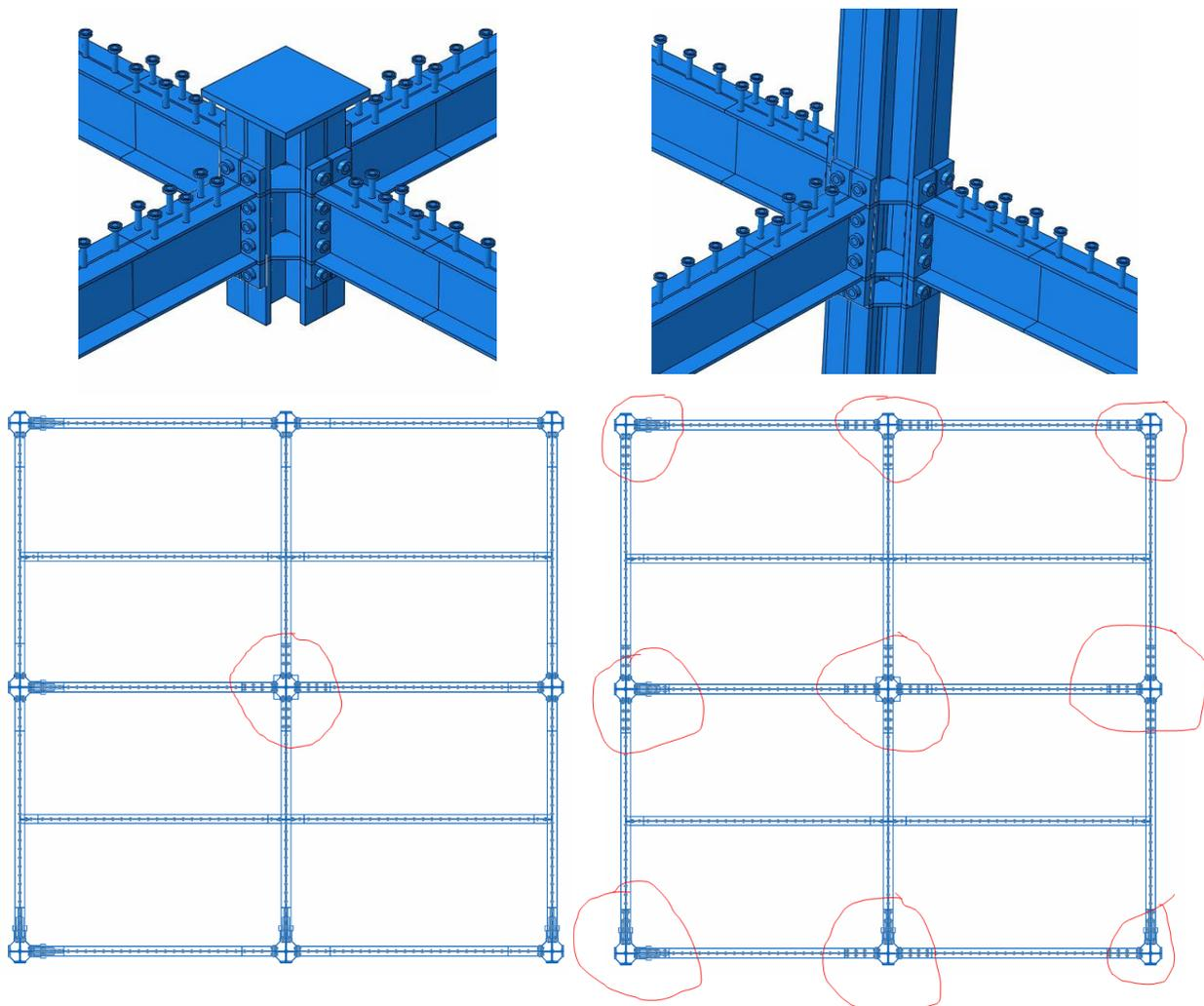
Figure 5.1 Number and spacing of shear connectors
