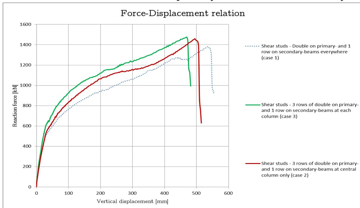
Figure 5.2 Force-Displacement relation for case 1, case 2 and case 3 (shear studs)
