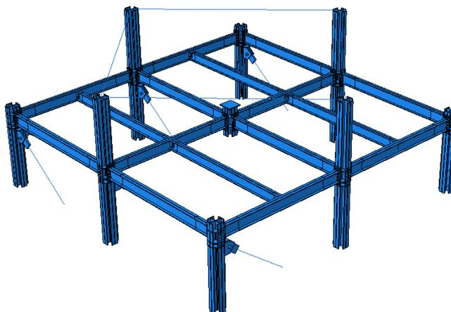
All the structural members and parts were modeled just how they will be in the sub-assembly for the experimental testing (Figure 4.57).
