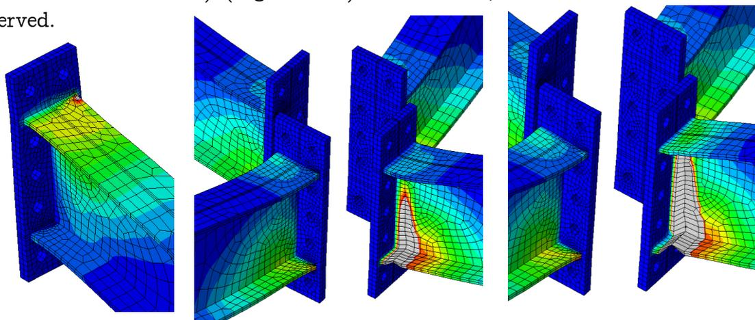
Figure 4.44 Development of plastic hinges at the end of beams
