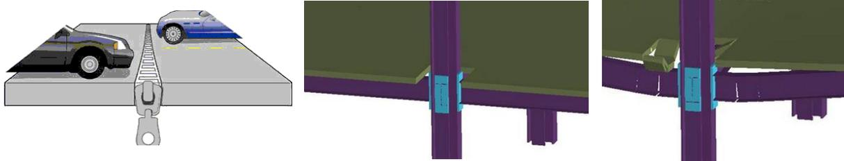
Figure 4.65 Zipper failure of shear connectors in concrete slab (Marginean et al, 2013)
