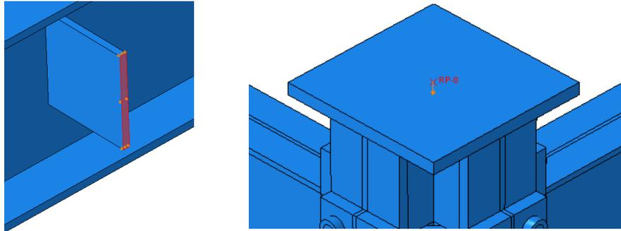
Figure 4.30 Boundary condition modeling and application of the displacement based loading. Full analysis was created, using multiple processors (4) and single precision. In Figure 4.30 it can be observed the deformed shape of the frame and the PEEQ (equivalent plastic strain) distribution within the structure.
