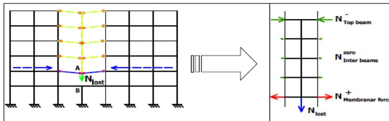
Figure 1.16 Distribution of the membrane forces in the directly affected part (Hai, 2009)
