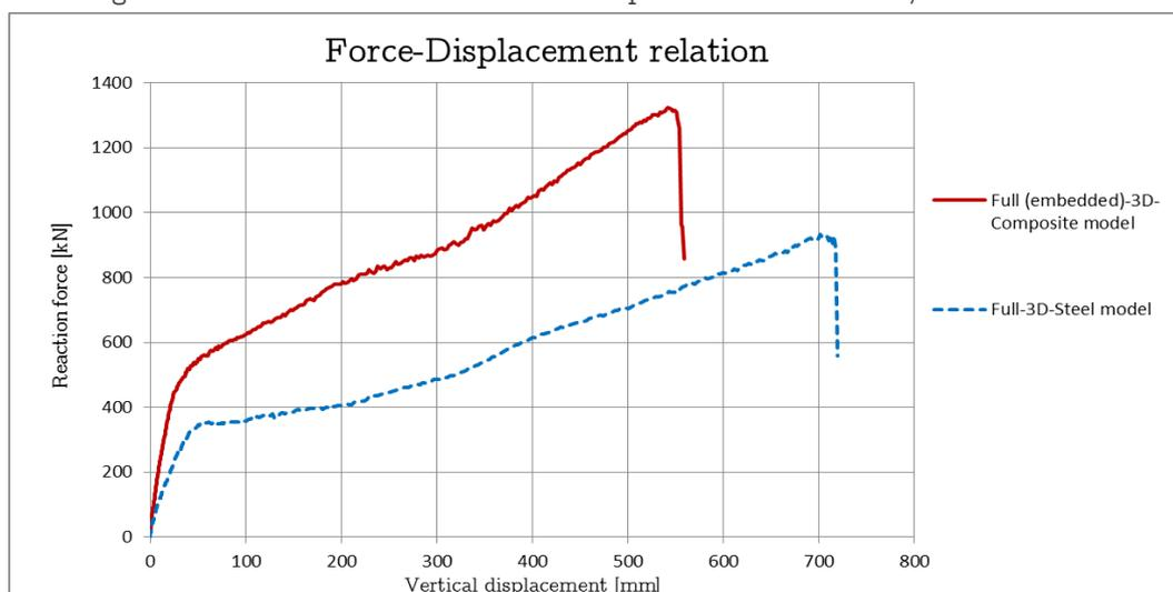
Figure 4.73 Comparison of Force-Displacement curve for full 3D steel model and 3D composite model
