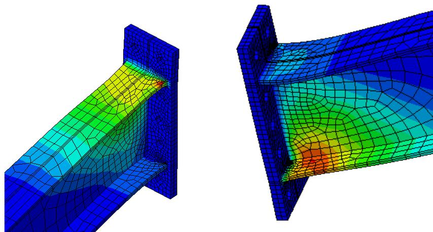
Figure 4.33 Development of plastic hinges at the end of beams
