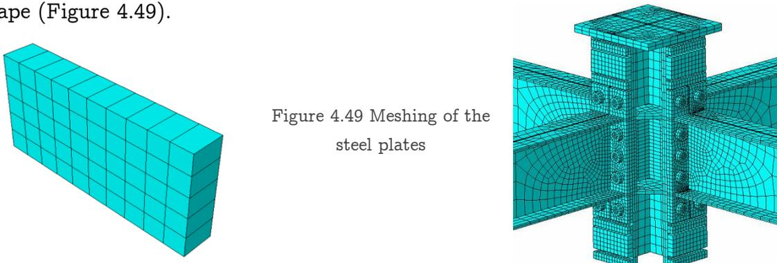
Figure 4.49 Meshing of the steel plates
