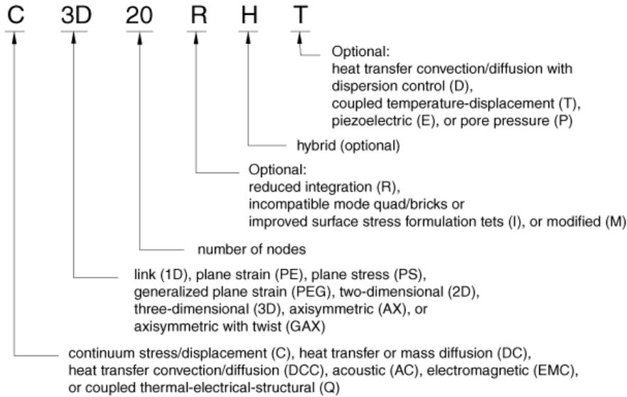
Figure 4.16 Name convention of solid elements (Abaqus user manual)
