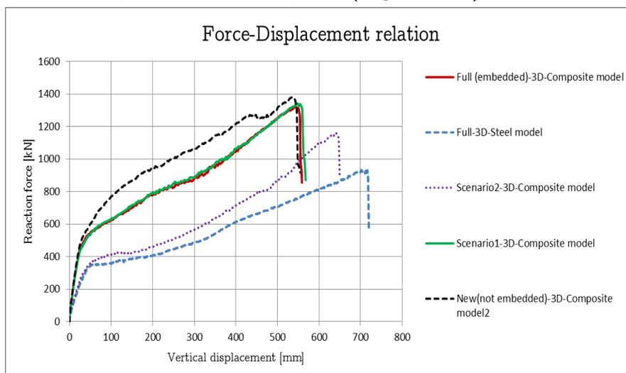
Figure 4.79 Comparison of Force-Displacement curve for full 3D steel model, full 3D composite model, Scenario 1 3D composite model, Scenario 2 3D composite model and the new(not embedded) 3D composite model
