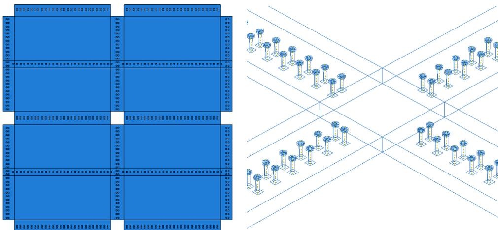
Figure 4.69 Division of the concrete slab inferior surface into smaller surfaces
