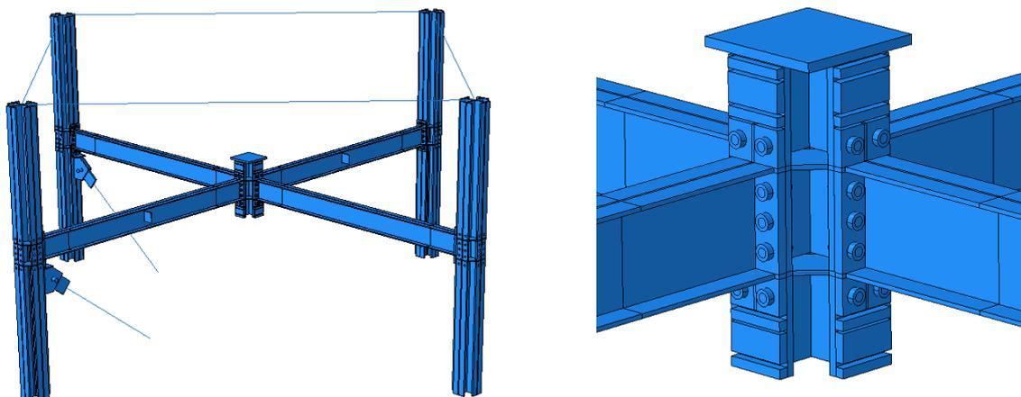
Figure 4.48 Constrained rotation tendency of the loaded column (3D model)
