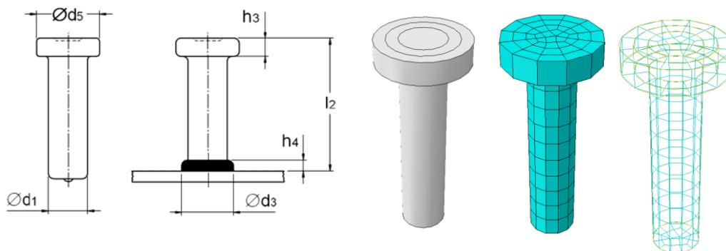
Figure 4.66 Shear connector modeled in Abaqus
