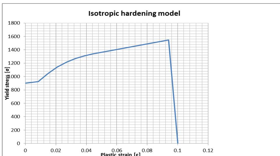
Figure 4.13 Isotropic hardening model data used for defining the nonlinear plastic behavior of steel
