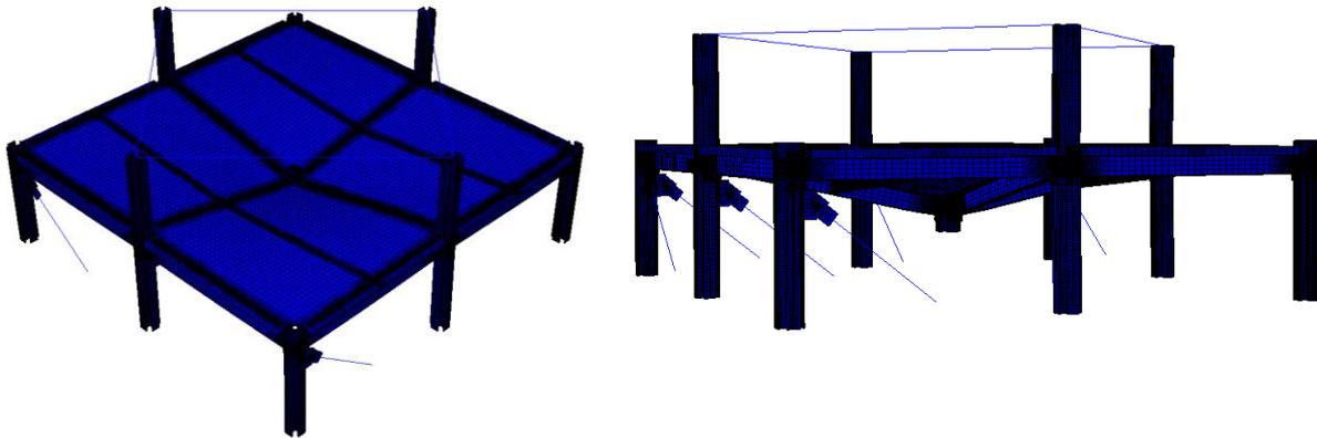
Figure 4.70 Deformed shape of the structure
