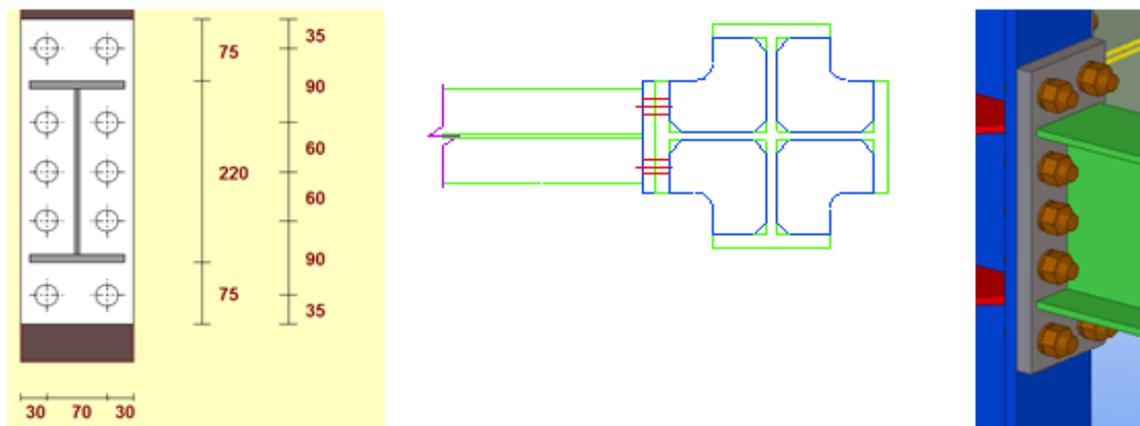
Figure 3.12 Column-to-beam connection configuration
