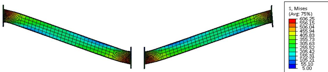
Figure 4.34 Stresses in the beams at a displacement of 720 mm, load of 437 kN
