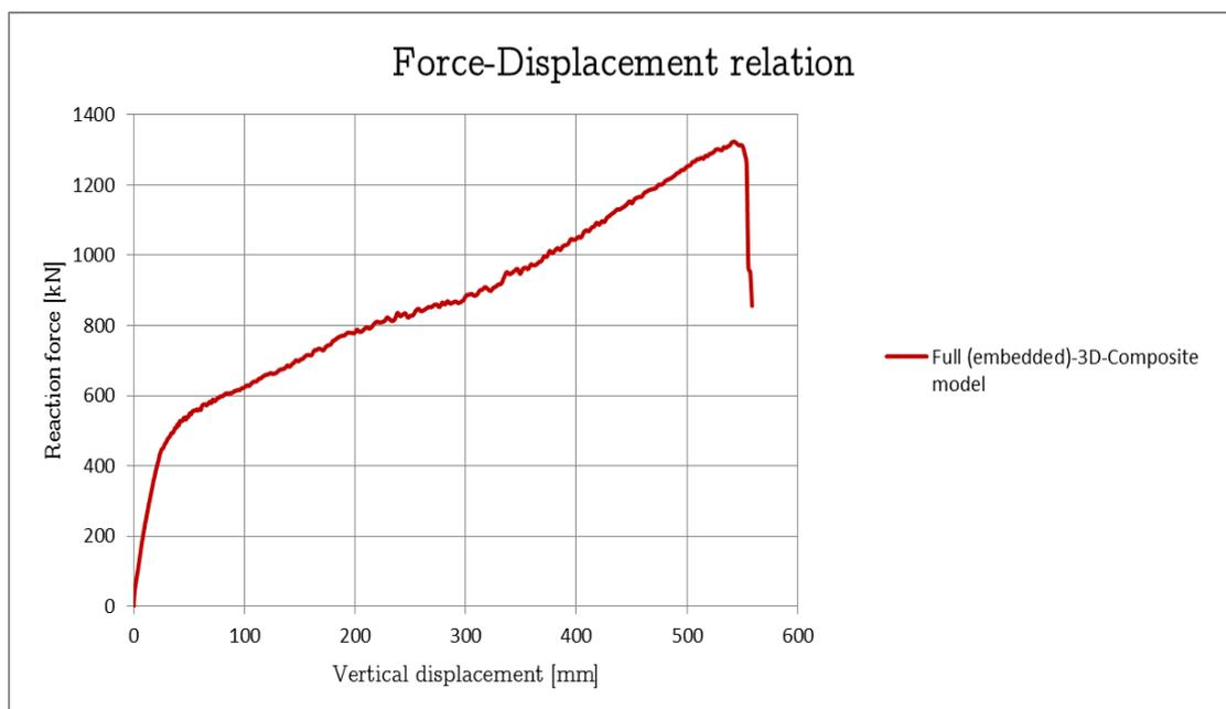
Figure 4.71 Force-Displacement curve for the 3D-model considering the composite action
