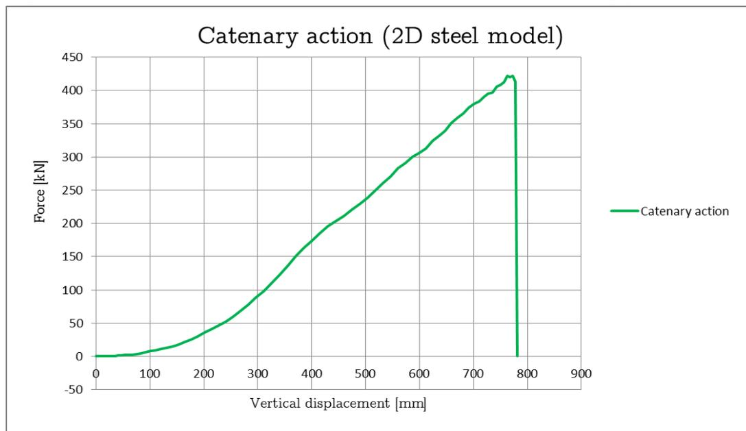
Figure 4.83 Contribution of the catenary action for the total applied loading (2D steel model)
