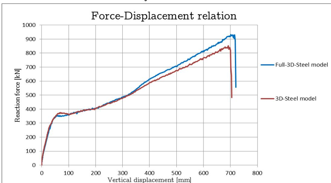
Figure 4.60 Comparison of Force-Displacement relation for the full 3D-model and simple 3D model
