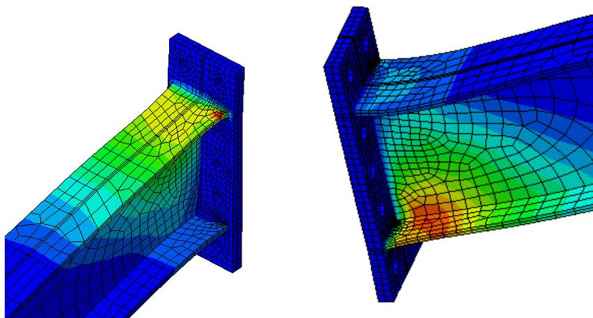
Figure 4.33 Development of plastic hinges at the end of beams
