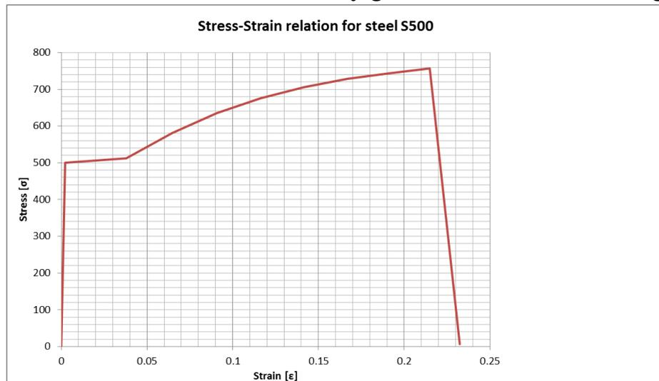
Figure 4.10 Stress-Strain relation of steel S500
