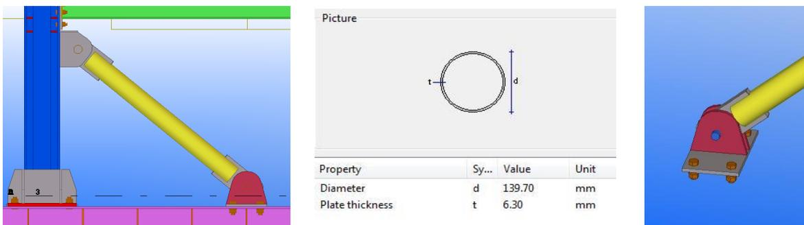
Figure 3.8 Bracing system cross-sectional characteristics
