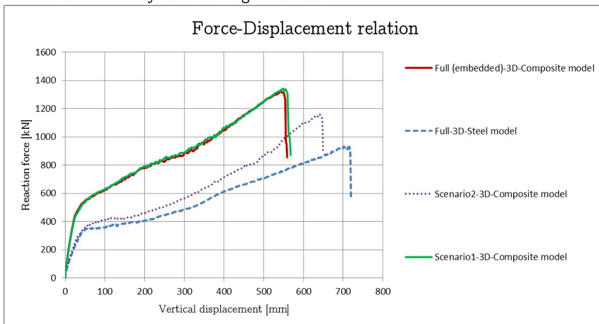
Figure 4.75 Comparison of Force-Displacement curve for full 3D steel model, full 3D composite model, Scenario 1 3D composite model and Scenario 2 3D composite model
