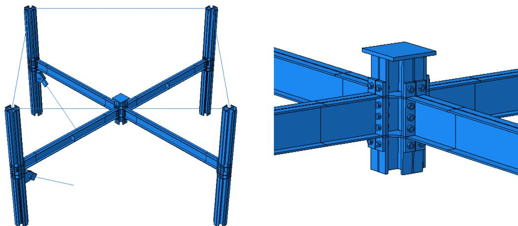
Figure 4.37 Finite element model of the 3D sub-assembly
