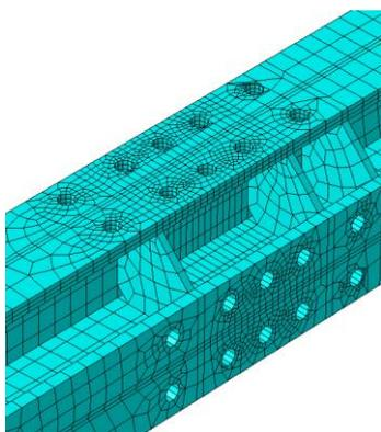
Figure 4.19 Exterior column mesh at the level of the connection
