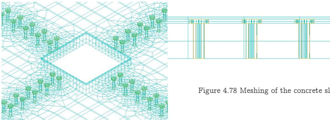
Figure 4.78 Meshing of the concrete slab
