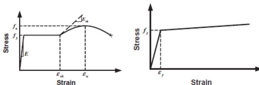
Figure 4.5e Elasto-perfectly plastic model with strain hardening (Eurocode)
