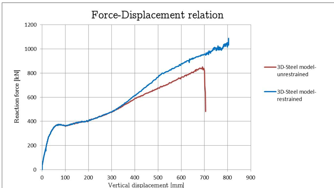
Figure 4.53 Force-Displacement curve for the 3D-model (restrained column case)
