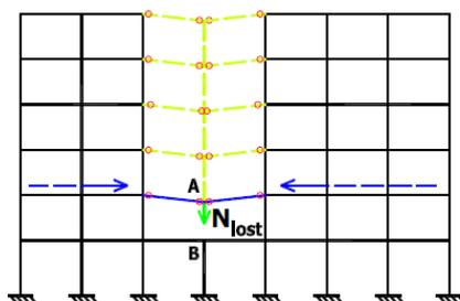
Figure 4.1 Catenary action in the case of  $N_{lost}^{PL,Rd} < N_{design}$  (Hai, 2009)
