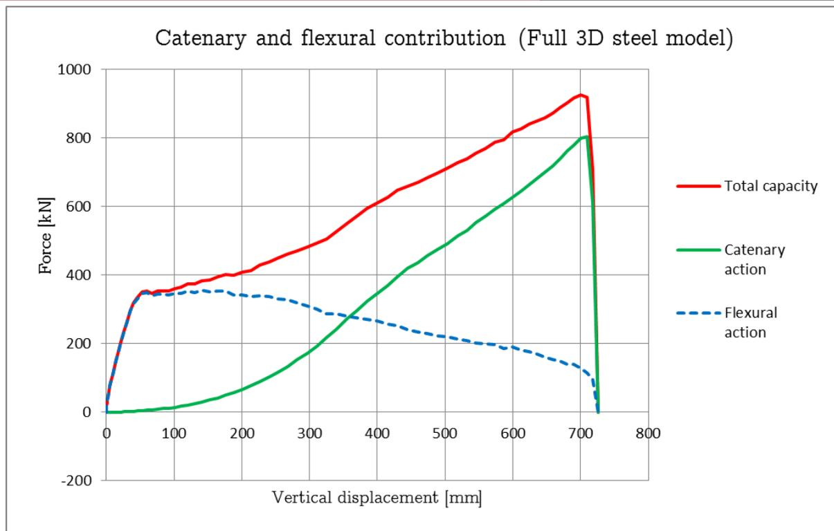
Figure 4.86 Catenary and flexural action for the Full 3D steel model
