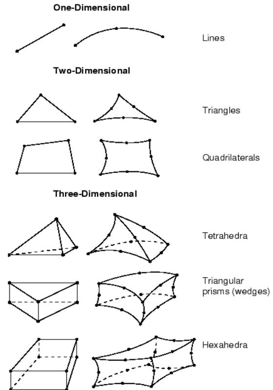
Figure 4.17 Mesh element shapes (Abaqus users manual)
