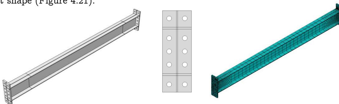
Figure 4.21 Primary-beam model
