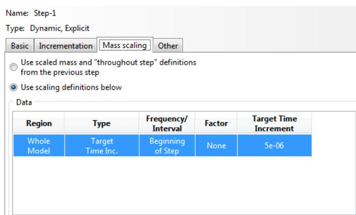
Figure 4.29 Mass scaling of the model
