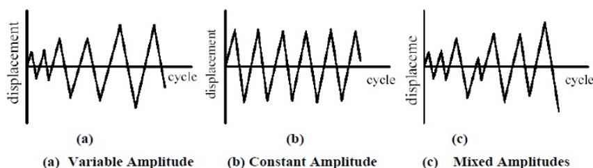
Figure 4.3 Various types of loading histories in quasi-static cyclic tests ([www.engpedia.com](http://www.engpedia.com))
