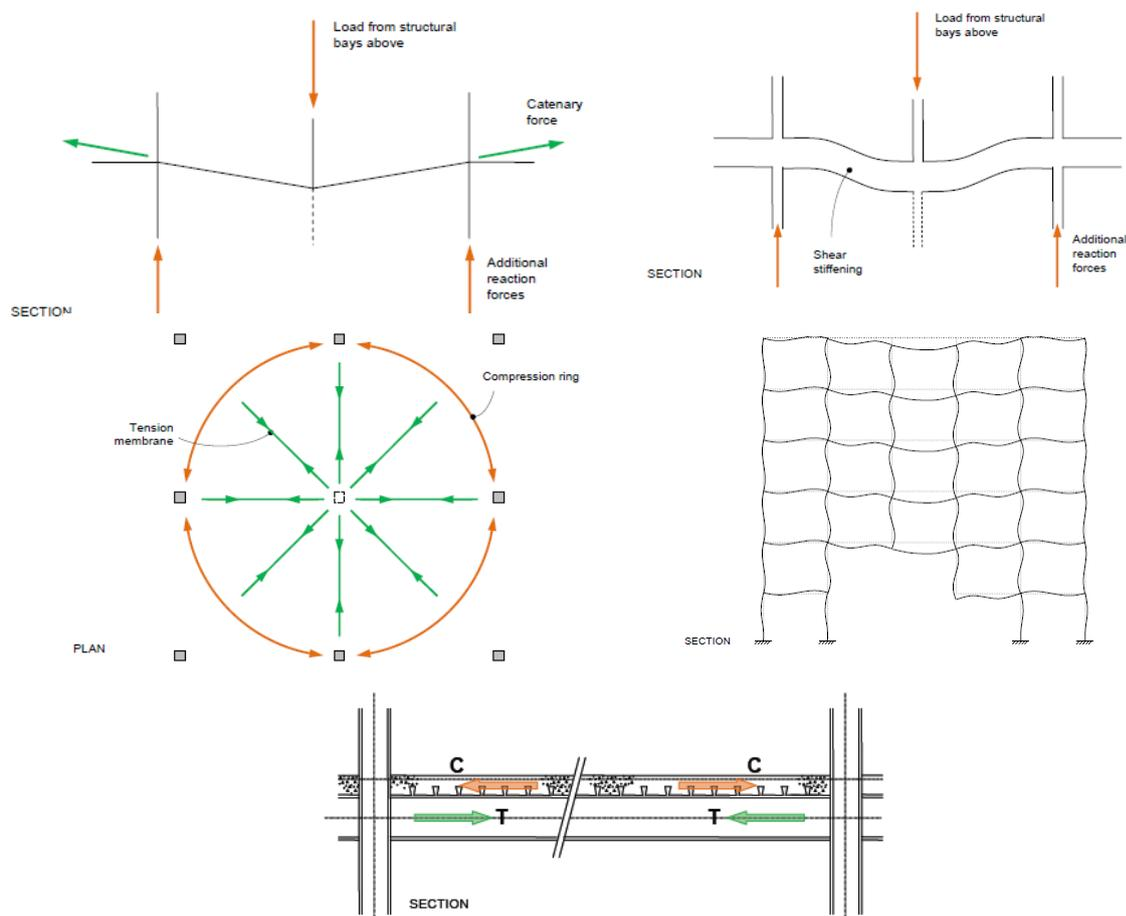
Figure 1.20 The five mechanisms fundamental to robustness problem (Cormie, 2009)
