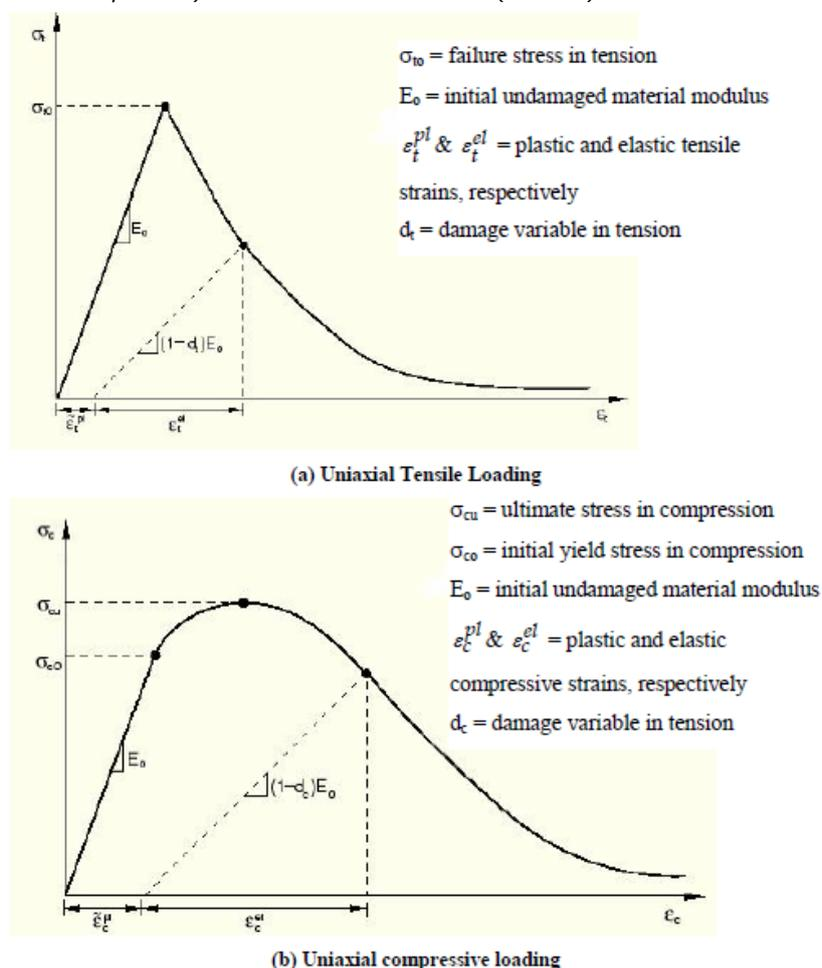
Figure 4.2a Uniaxial tensile and compressive model for concrete (Abaqus users manual and EC2)
