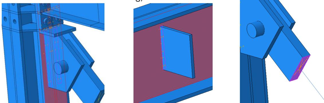
Figure 4.27 Tie constraint for the bracing, end-plate connection modeling
