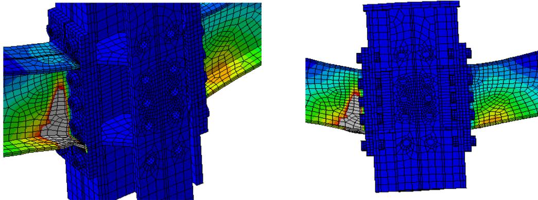
Figure 4.35 Failure of the structure at a displacement of 770 mm, load of 470 kN
