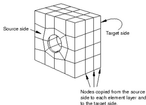
Figure 4.25 Sweep mesh technique (Abaqus user manual)
