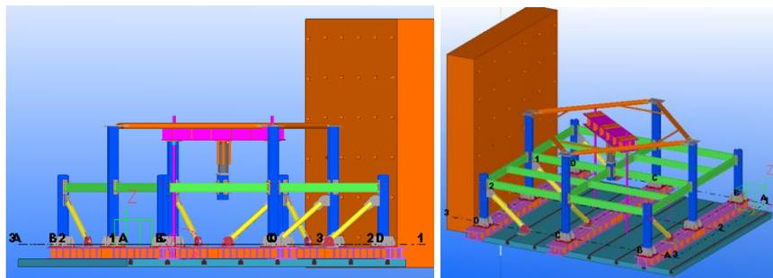
Figure 4.2 Test set-up of the sub-assembly for the experiment
