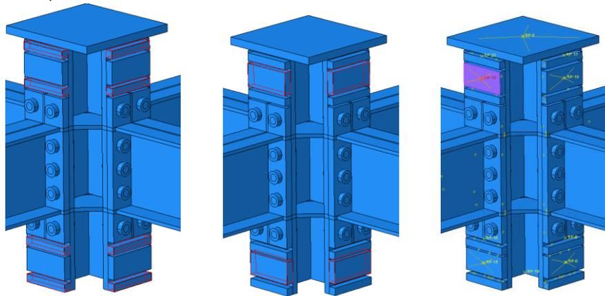
Figure 4.50 Constraints on the column-to-steel plate connection
