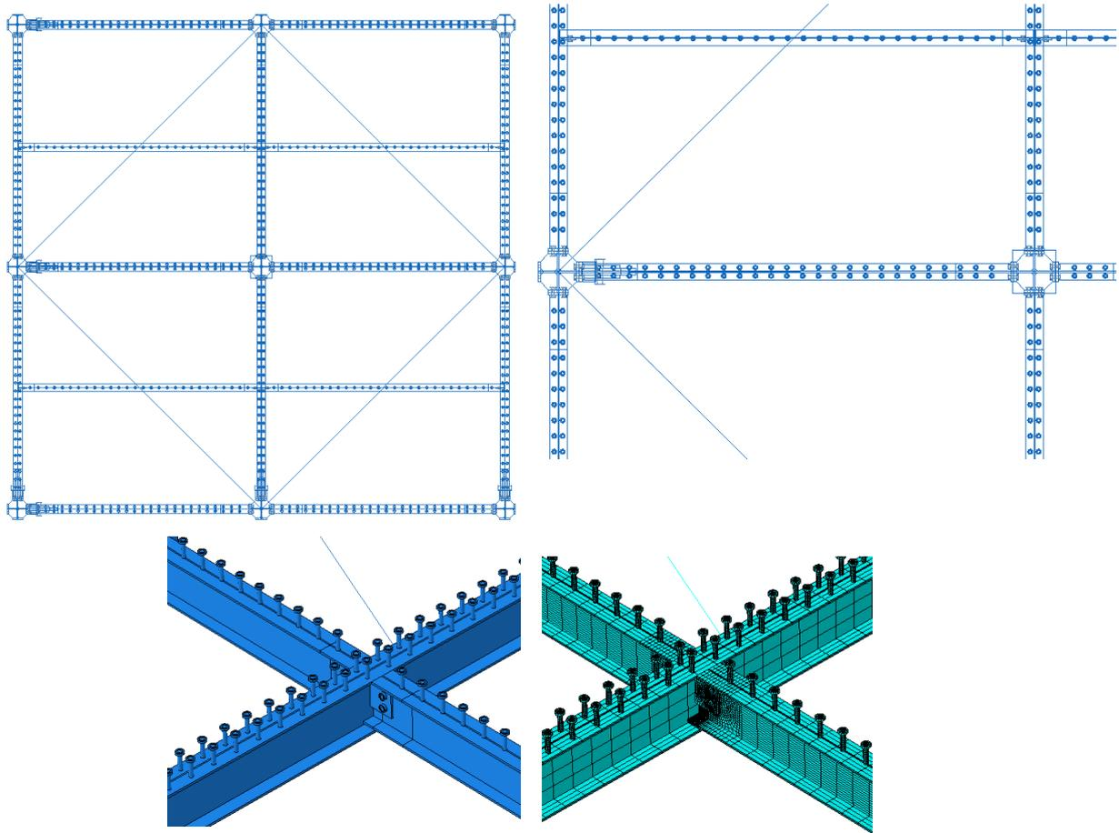
Figure 4.67 Spacing of shear connectors in the model
