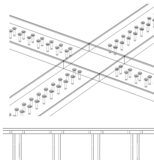
was equal to the dimensions of the shear stud. For meshing the slab two techniques were used: structured mesh for the eight central slab panels and sweep mesh (using advancing front algorithm) for the parts where the holes have been defined (Figure 4.78). Before meshing the concrete slab it was necessary to partition the thickness of the slab into several parts, according to the shape of the hole (shear connector) (Figure 4.77).
