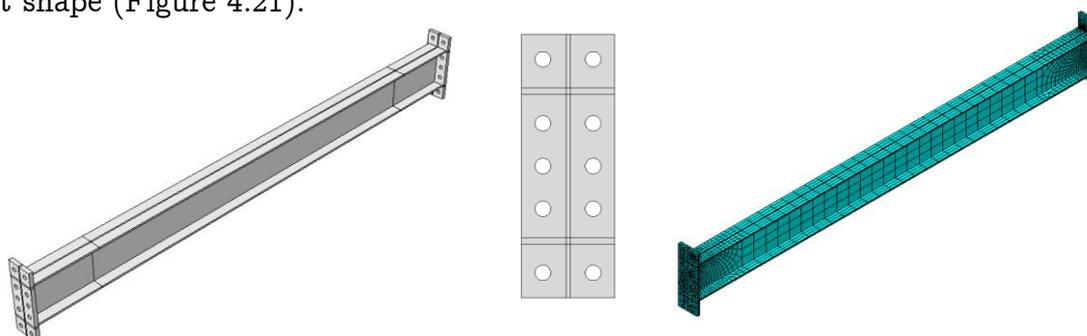
Figure 4.21 Primary-beam model
