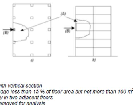
Figure 2.1 Recommended limit of acceptable damage in EN 1991-1-7:2006
