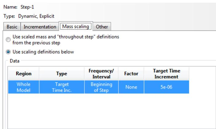
Figure 4.29 Mass scaling of the model
