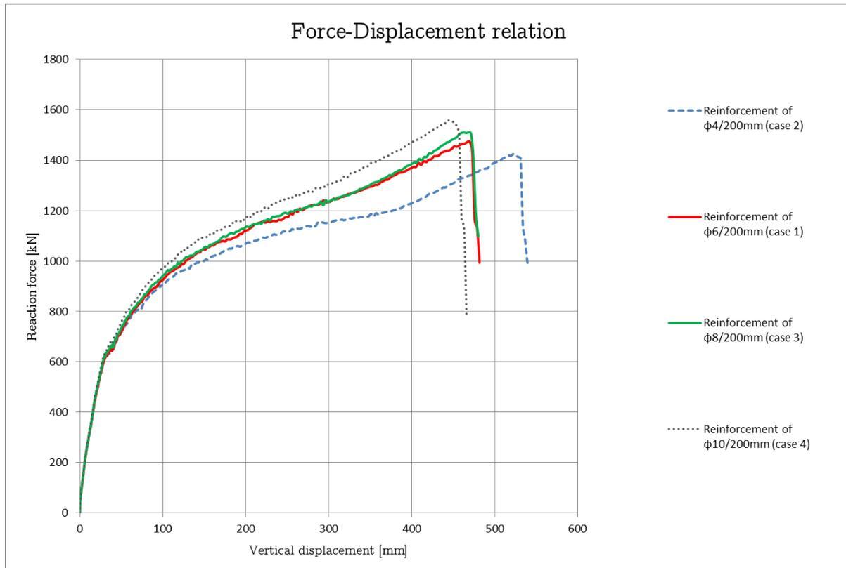
Figure 5.5 Force-Displacement relation for case 1, case 2, case 3 and case 4 (reinforcement ratio)
