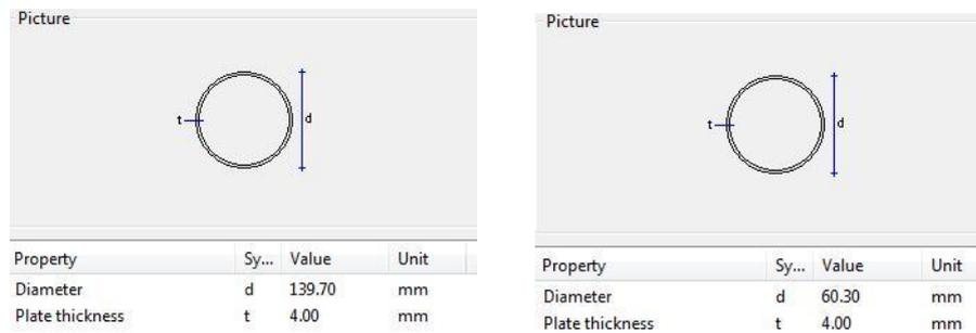
Figure 3.7 CHS cross-sectional characteristics
