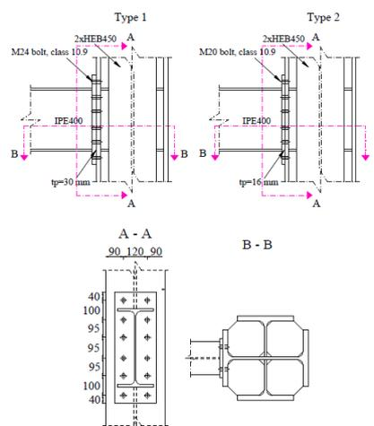
Figure 3.4 Connection details of beam-to-column (Marginean et al, 2013)
