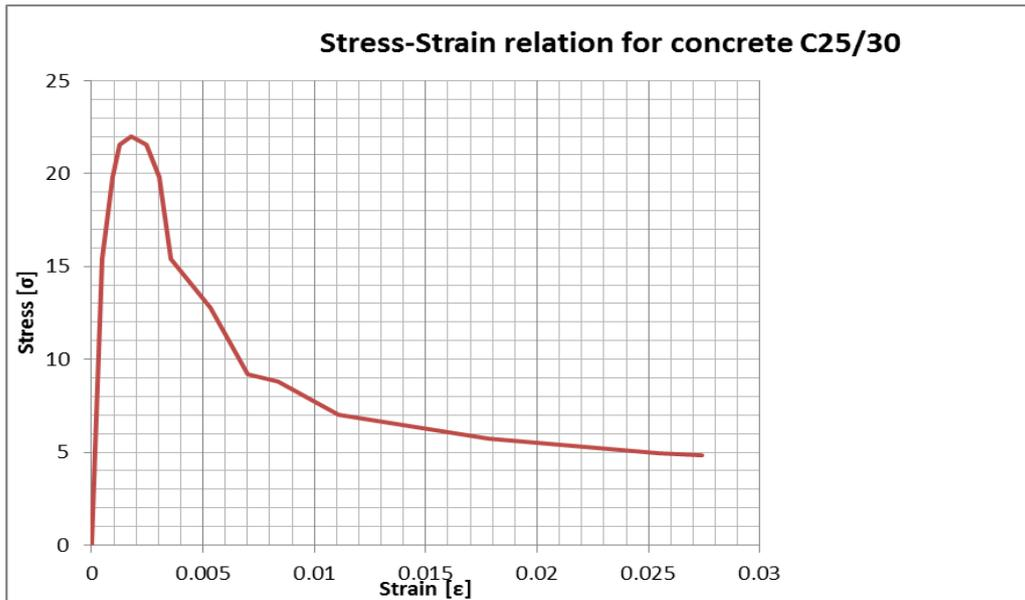
Figure 4.8 Stress-Strain relation of concrete C25/30 (compressive behavior)
