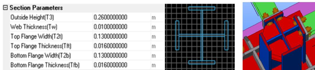
Figure 3.9 Column cross-sectional characteristics
