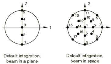
Figure 4.63 Circular cross-section from standard beam section library (Abaqus user manual)
