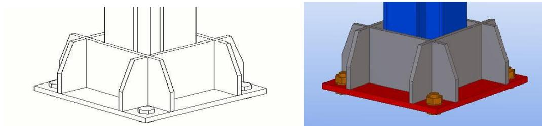
Figure 3.11 Column base connection configuration
