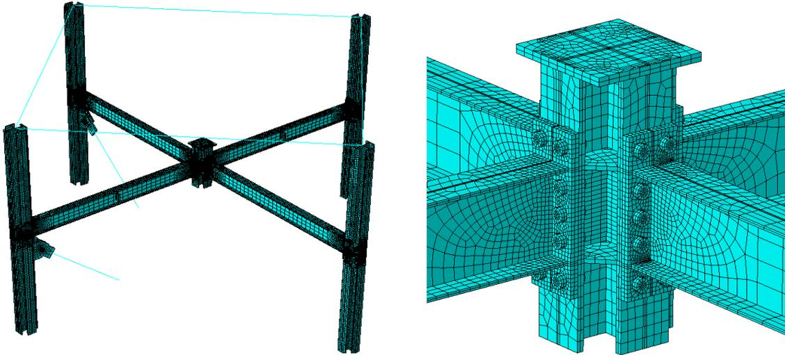
Figure 4.39 Mesh defined for the 3D model
