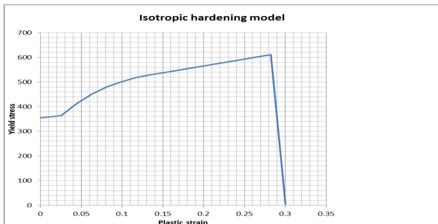
Figure 4.7 Isotropic hardening model data used for defining the nonlinear plastic behavior of steel
