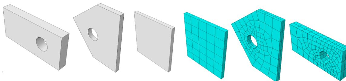
Figure 4.26 End-plate and stiffener models
