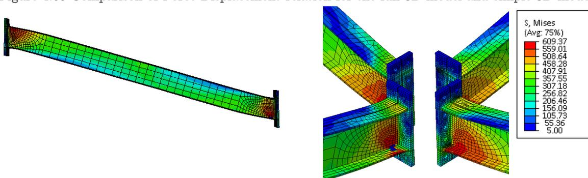
Figure 4.61 Stresses in the beams at a displacement of 701 mm, load of 932 kN
