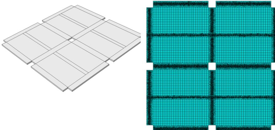
Figure 4.68 Modeling of the concrete slab in Abaqus
