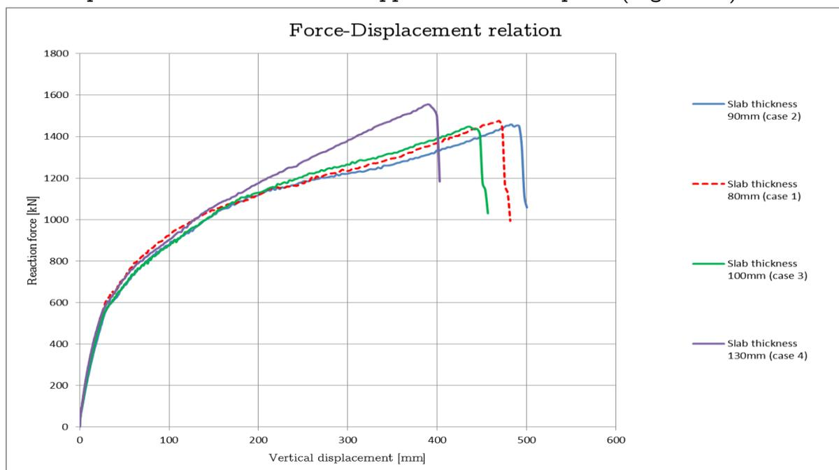
Figure 5.4 Force-Displacement relation for case 1, case 2, case 3 and case 4 (slab thickness)
