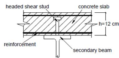
Figure 3.2 Cross-section of composite secondary beam (Marginean et al, 2013)
