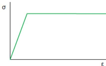
Figure 4.5d Simplistic linear elastic-perfectly plastic material response (Arup)
