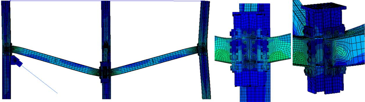
Figure 4.47 Rotation tendency of the loaded column (3D model)
