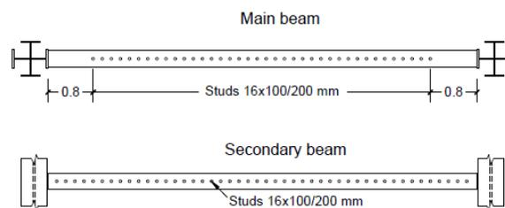
Figure 3.3 Spacing of connectors for main and secondary beams (Marginean et al, 2013)
