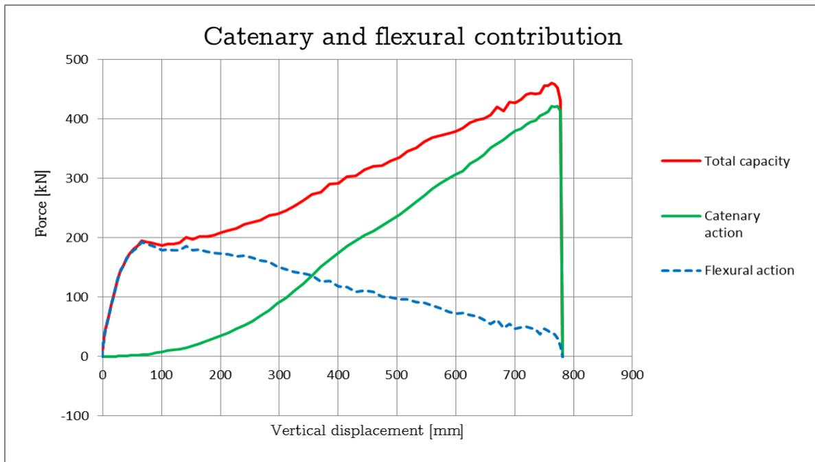
Figure 4.85 Catenary and flexural action for the 2D steel model
