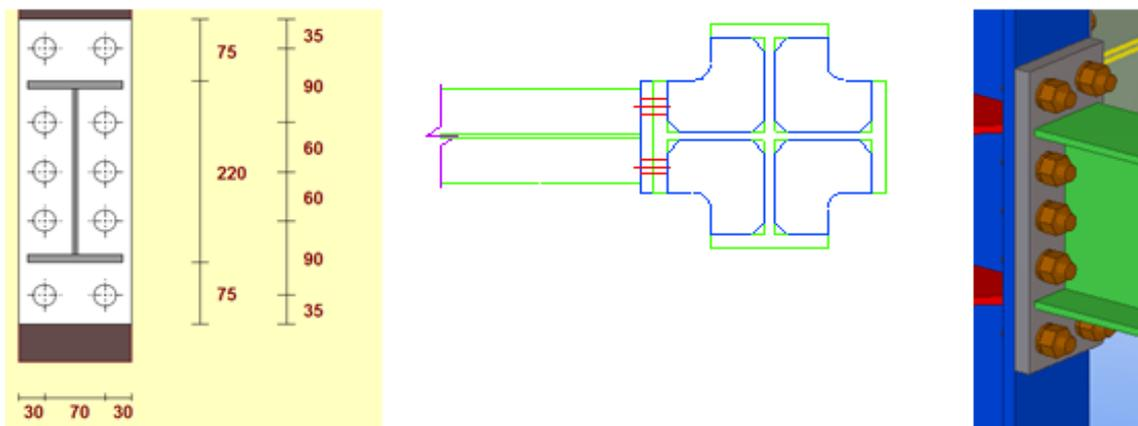
Figure 3.12 Column-to-beam connection configuration
