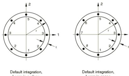
Figure 4.22 Pipe cross-section from standard beam section library (Abaqus user manual)
