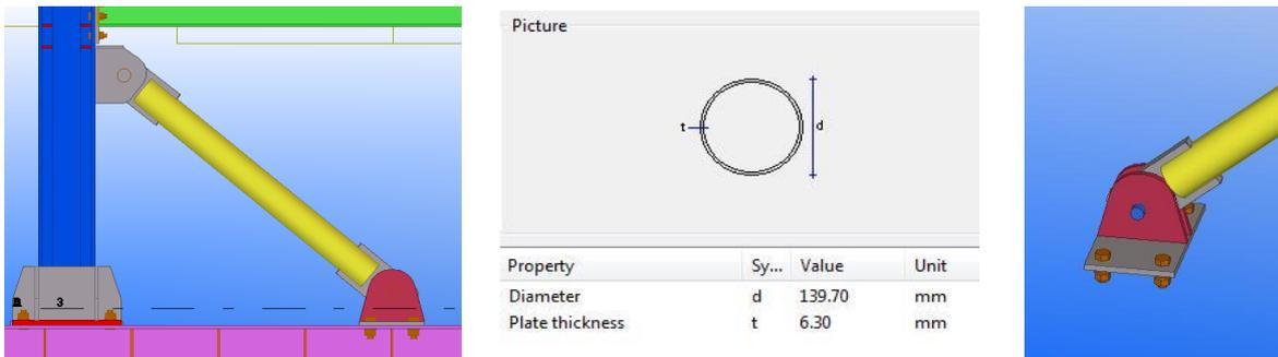
Figure 3.8 Bracing system cross-sectional characteristics
