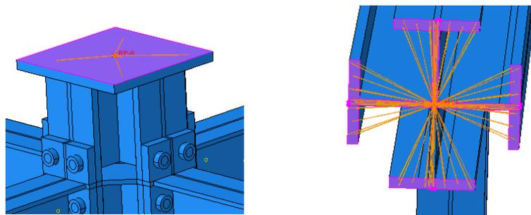
Figure 4.28 Coupling into control points the motion of the top-plate and column base
