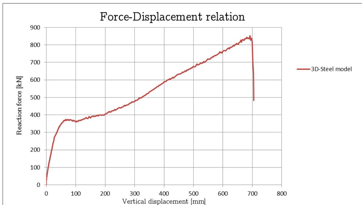
Figure 4.43 Force-Displacement curve for the 3D-model
