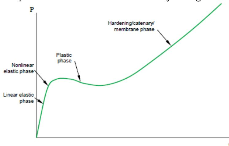
Figure 4.32a Typically nonlinear static response of the damaged structure (Arup)
