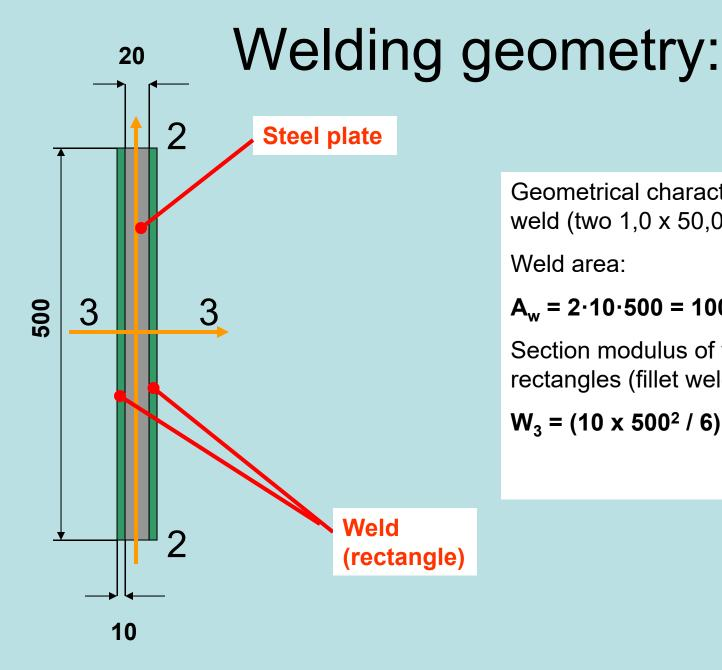
Geometrical characteristics of the fillet weld (two 1,0 x 50,0 rectangles):
