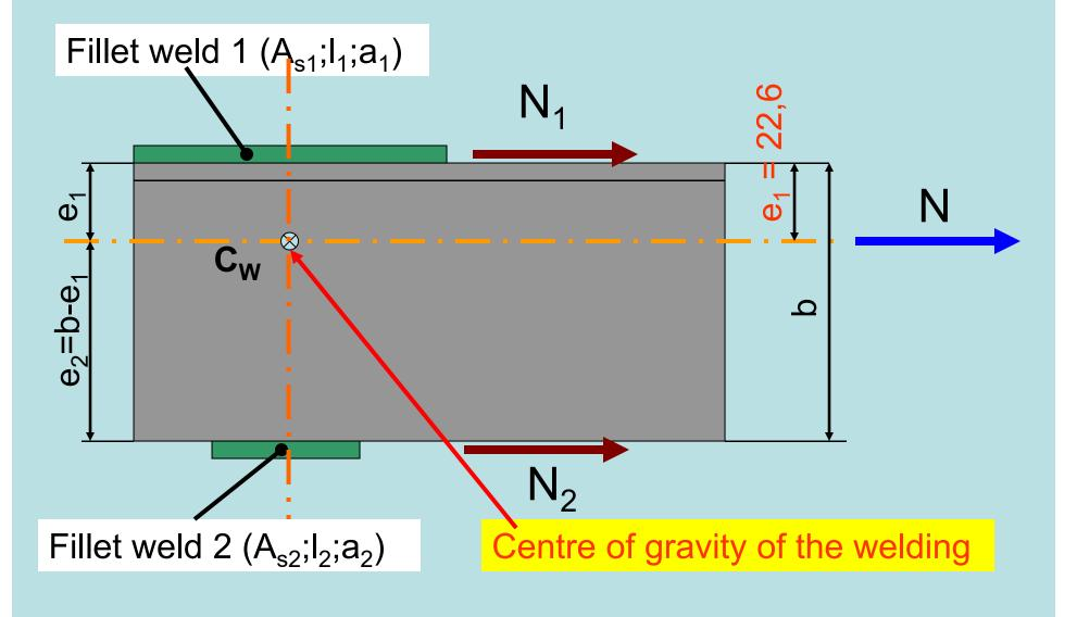
Condition for the two unequal welds to have the centre of gravity on member axis:
