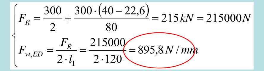
Calculation of the design shear strength of the weld:
