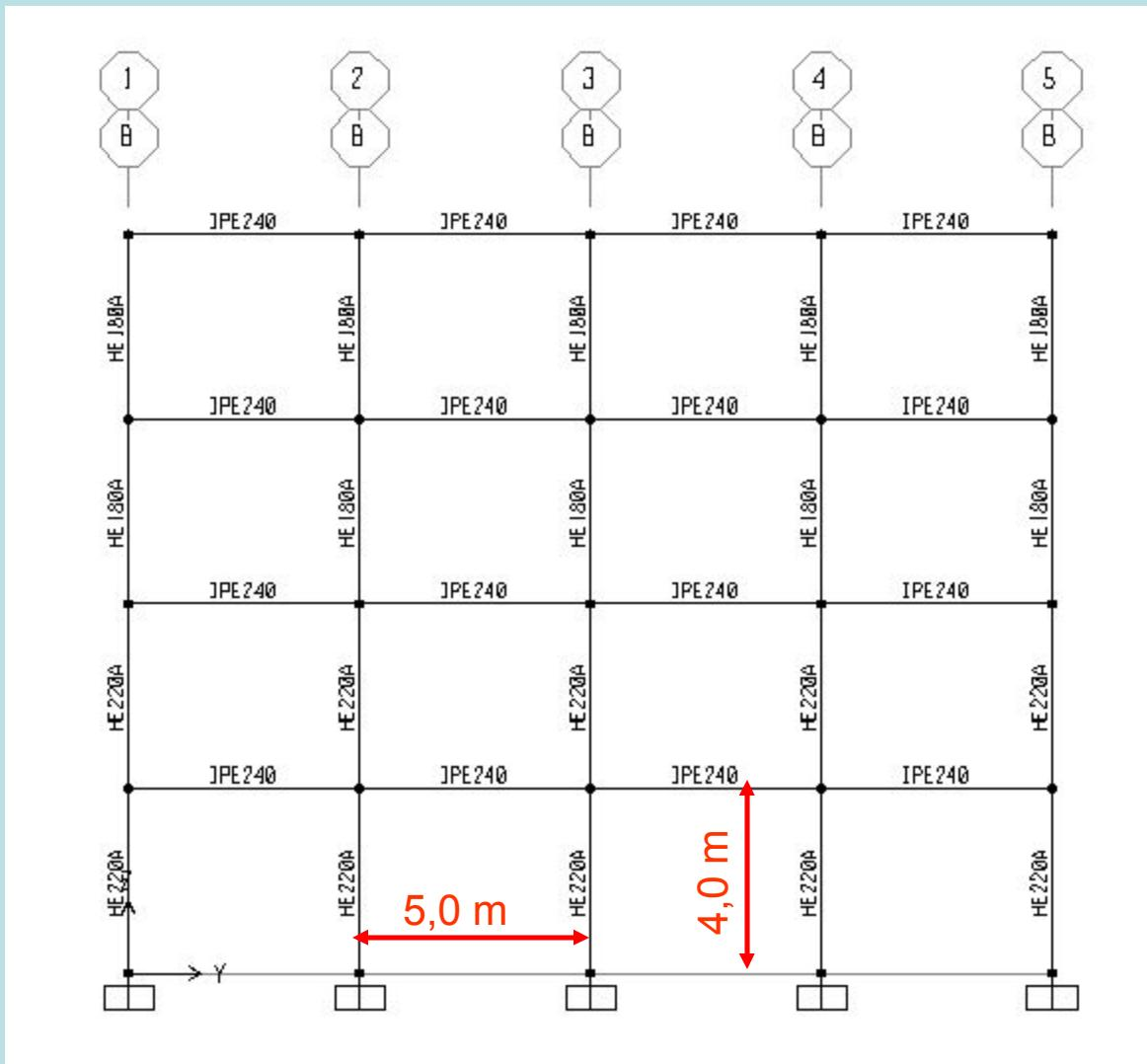
Labels of the columns for longitudinal frame
