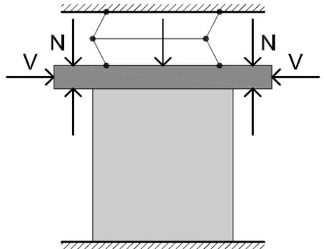
Type A setup with pantograph
