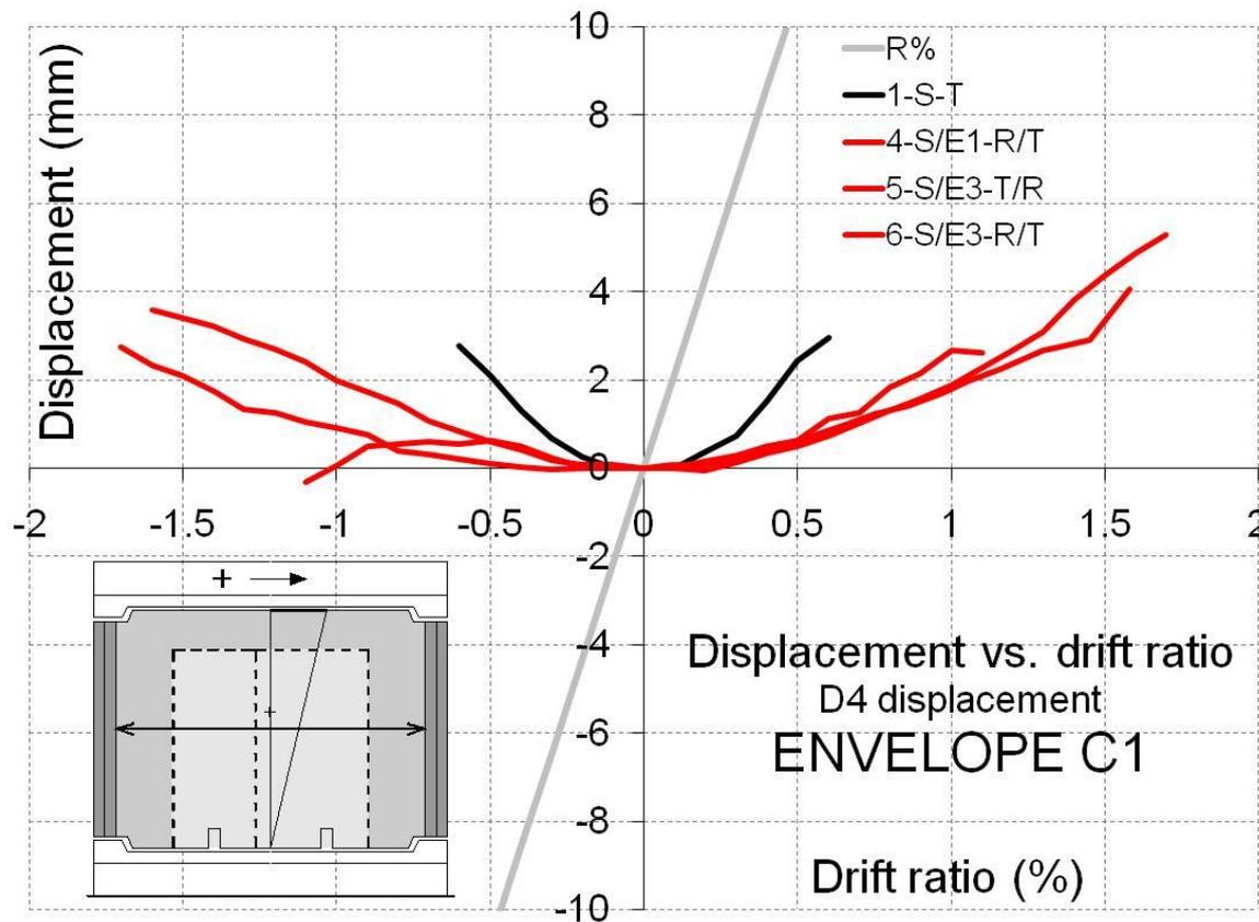
Shear characteristic horizontal lengthening at the mid-height of the walls.
