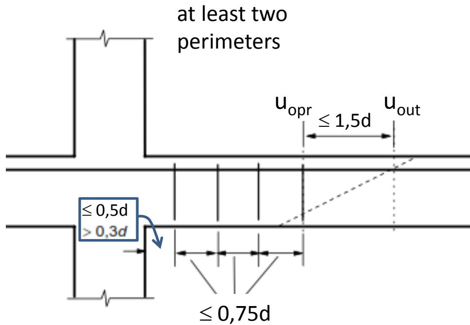
$$s_r \leq 0.75d = ? \text{ mm} \quad \rightarrow \quad s_r = ? \text{ mm}$$
