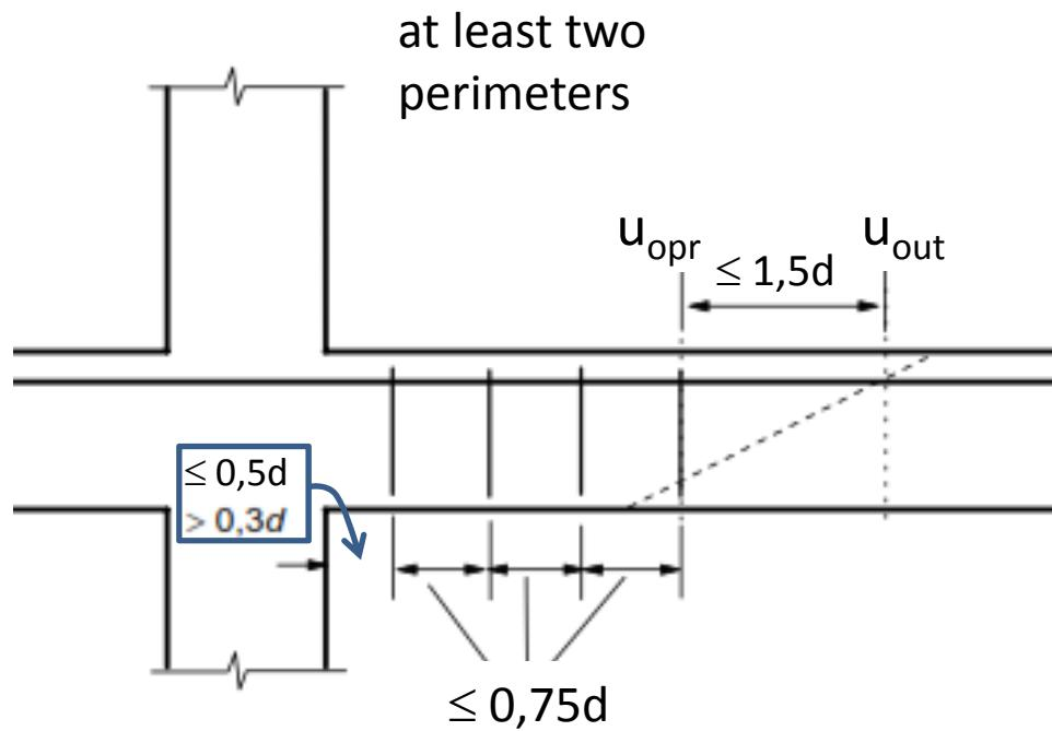
$$s_r \leq 0.75d = 170 \text{ mm} \quad \rightarrow \quad s_r = 150 \text{ mm}$$
