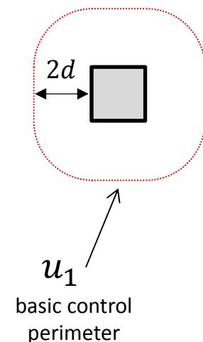
$$\begin{aligned} \rightarrow \quad & \nu_{Ed,u_1} = \beta \frac{V_{Ed}}{u_1 \cdot d} = ? \text{ MPa} \\ \rightarrow \quad & \nu_{Rd,c} = C_{Rd,c} k (100 \rho_l f_{ck})^{1/3} = ? \end{aligned} \quad \left. \right\} \quad \rightarrow \quad \nu_{Ed,u_1} <?> \nu_{Rd,c}$$
