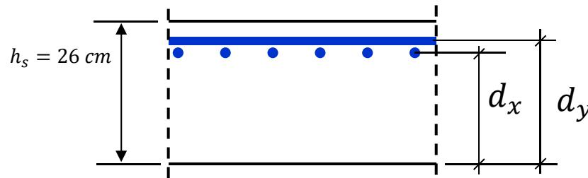
$$c_x = 20 + \frac{14}{2} = 27 \text{ mm} \quad \rightarrow \quad d_x = 260 - 27 = 233 \text{ mm}$$
