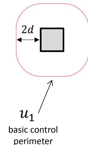
$$\begin{aligned} \rightarrow \quad & \nu_{Ed,u_1} = \beta \frac{V_{Ed}}{u_1 \cdot d} = 0.97 \text{ MPa} \\ \rightarrow \quad & \nu_{Rd,c} = C_{Rd,c} k (100 \rho_l f_{ck})^{1/3} = 0.57 \end{aligned} \quad \left. \right\}$$
