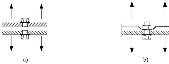
Possible failure modes for bolted connections in tension
