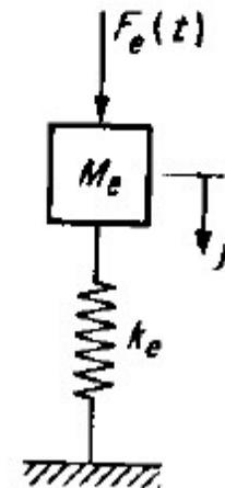
$F_e, K_e, M_e$  = characteristics of the equivalent SDOF system
