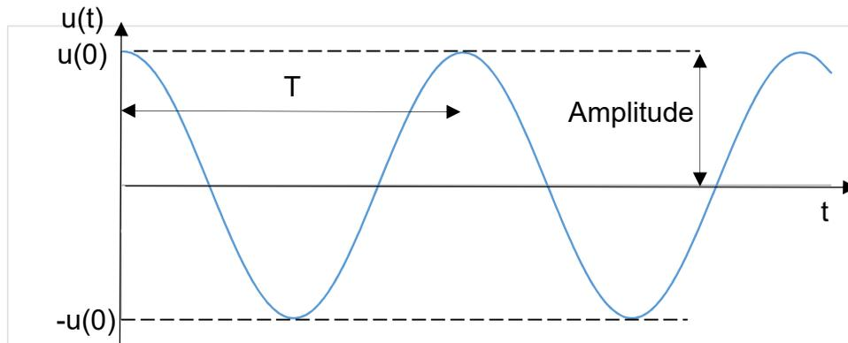
Free vibration of SDOF, undamped, initial displacement
