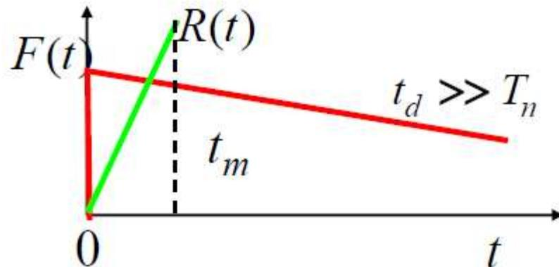
SDOF reaches  $u_m$  before load has any significant decay,  $F(t) \approx F$
