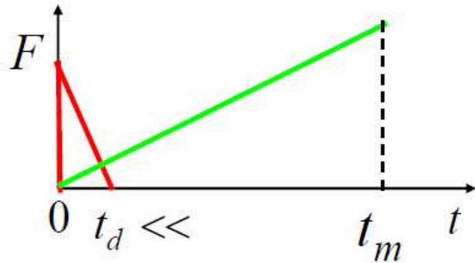
The load is applied so quickly even before the SDOF system has any movement. Response treated as free vibration with initial velocity due to impulse. Strain energy stored is the same as previous case.
