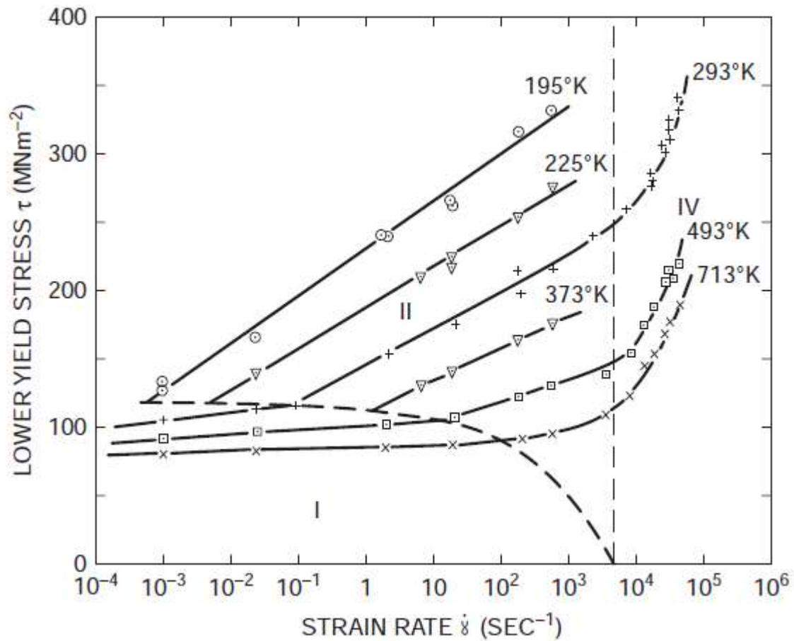
Effect of strain rate on mild steel
