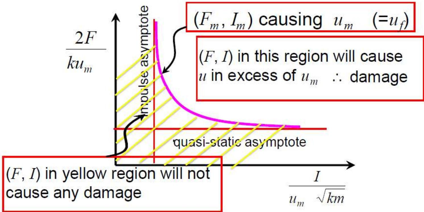
For a particular type of structure, diagrams are presented in absolute impulse (specific) vs. overpressure terms, for different damage ( $u_m$ ) levels
