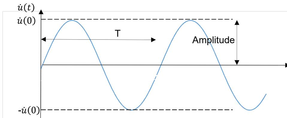
Free vibration of SDOF, undamped, initial velocity
