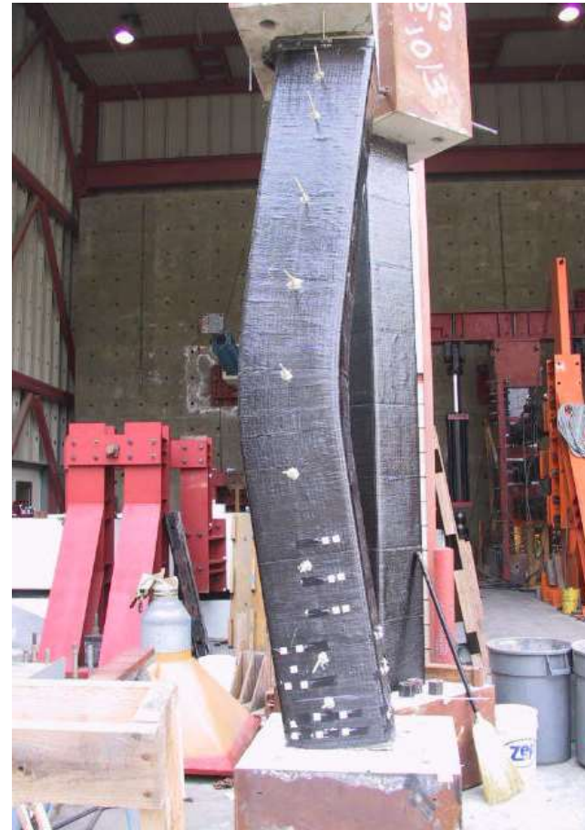
Reinforced concrete column without/with composite wrap
