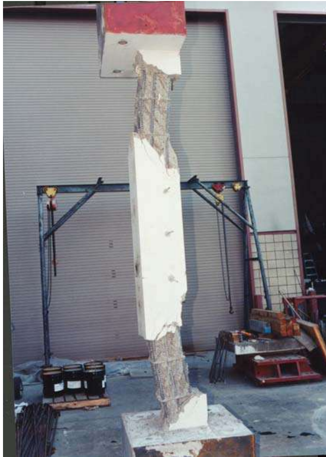
Reinforced concrete column without/with composite wrap
