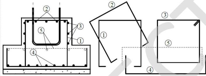
□ the **vertical reinforcement** (1 and 2 in the figure) results from eccentric axial check between the pillow and the foundation base;
