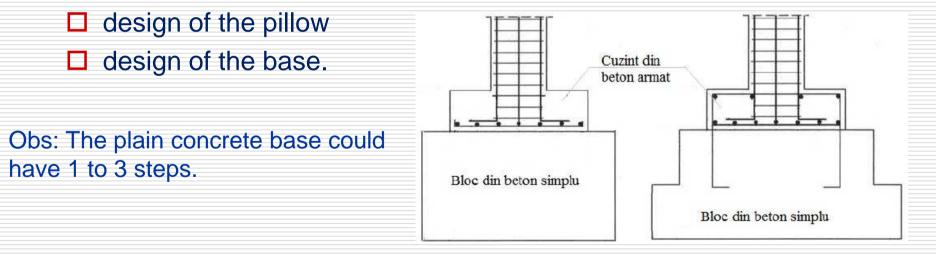
Obs: In order to obtain a horizontal footing level, a 5 to 10 cm equalizing concrete layer is cast (C8/10).
