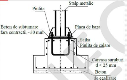
□ The minimum area of the base plate results from the condition:
