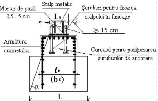
anchoring bolts (high diameter rods) are embedded in concrete, where they act as special reinforcements.
