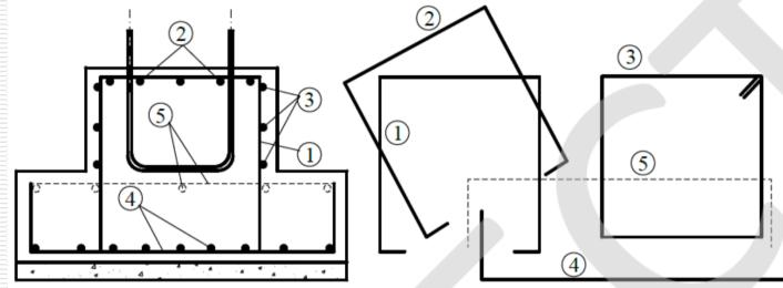
□ the **horizontal reinforcement** (no 3 in the figure) are disposed on the perimeter of the pillow;
