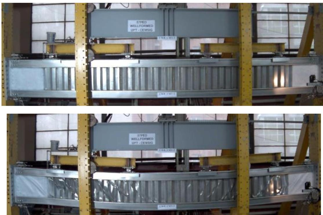
Figure 16: Beam CWB-CMT3 – before and after the testing.
