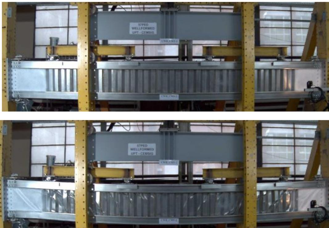
Figure 13: Beam CWB-CMT2 – before and after the testing.
