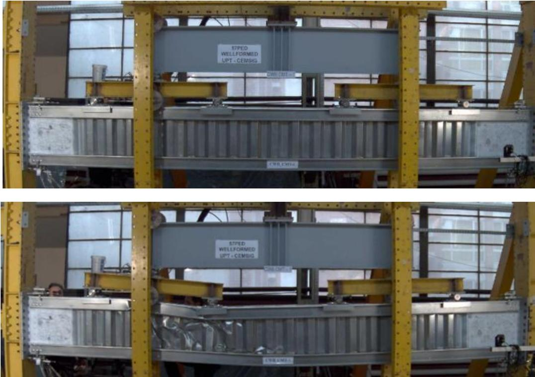
Figure 11: Beam CWB-CMT1 – before and after the test.
