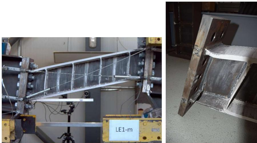
Fig. 11 – LE1 link deformation and failure at the end of LE1-M test
