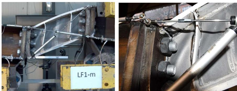
Fig. 6 – Failure mode of the end of LF1-M specimen
