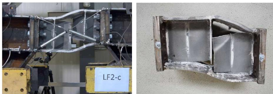
Fig. 8 –Failure mode of the LF2-C specimen
