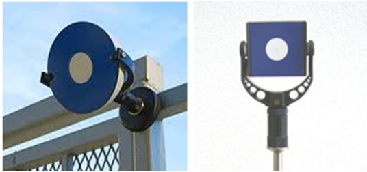
Figure 8 Circular planar target (6") and square planar target (3"x3")
