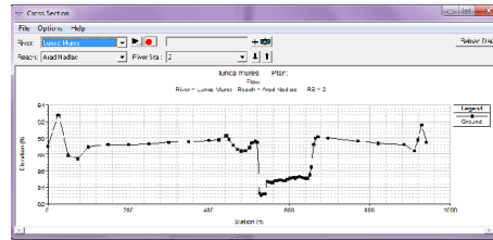
Fig. 7 Cross section through the Mures riverbed, Nadlac
