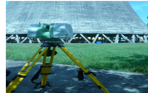
Fig.3 C10 ScanStation scanning system
