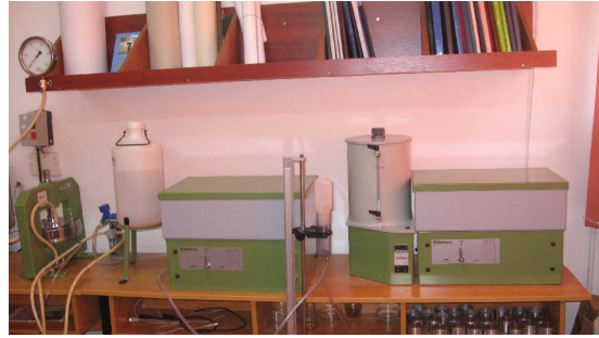
Foto.1 Experimental installation for the determination of the suction curve
