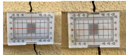
Figure 14. Photograph at the installation and final reading of benchmark C2
