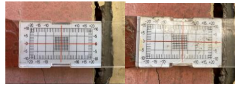
Figure 13. Photograph at the installation and final reading of benchmark C1
