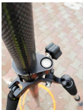
Figure 6. Leveling the receiver using the spherical level.
