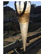
Figure 7. Sedimentation benchmark of fine particles from the extracted water
