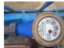
Figure 6. Flowmeter with the maximum accuracy of 0.0001 m 3
