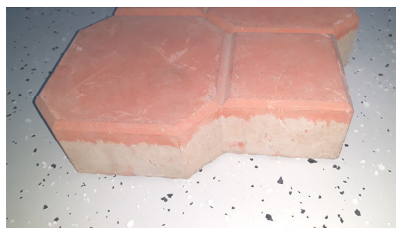
Figure 2. Photography with the pavement elements with ultrafine fly ash /2/
