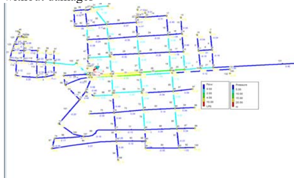
Figure.5. Pressure in distribution networks with damage
