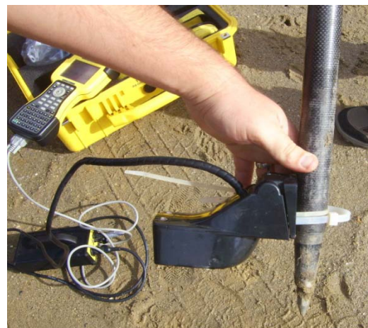
Figure 10 The connection between the GPS unit and the sonar
