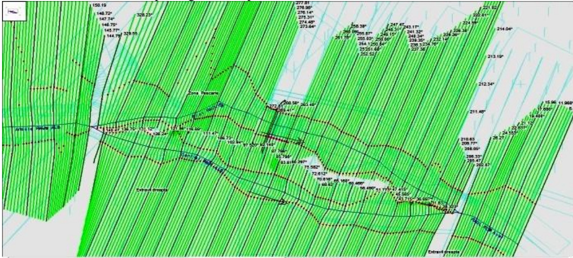
Figure 2.1 Layout of the numerical model with the overlaid catchment hydraulic structure [5]
