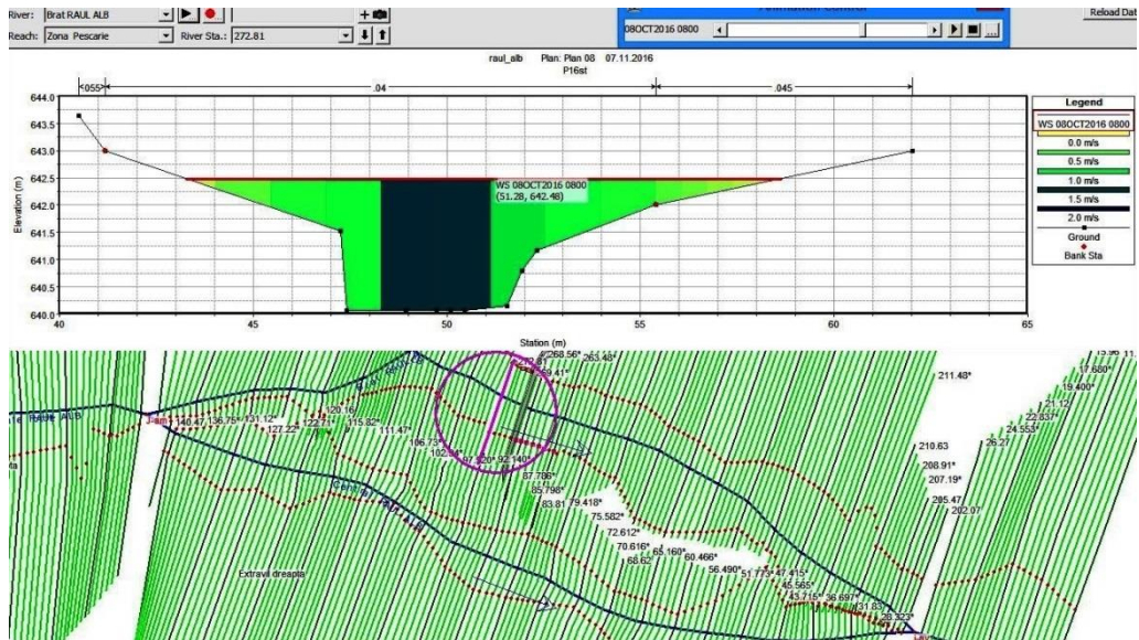
Figure 3.5a Flow scenario R4: water level and velocity in cross sections “144.79”- upstream of splitting point and “272.81-left”- upstream of overflow weir
