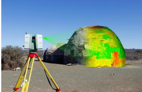
Figure 6. Terrestrial Laser Scanning System
