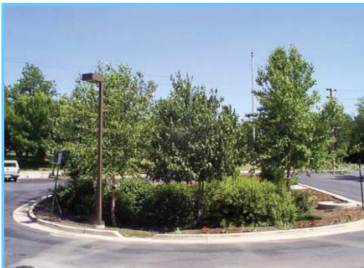
Fig. 7 Bioretention landscapes islands with curb cut to allow flows to enter [Coffman]
