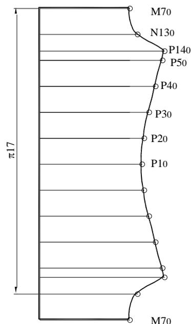
Fig. 3. Unfolding of the cylinder with inclined axis
