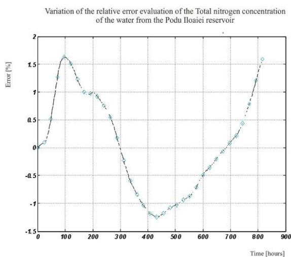
**Fig. 4-** Variation of the relative error of the Total nitrogen concentration of the water from the Podu Iloaiei reservoir
