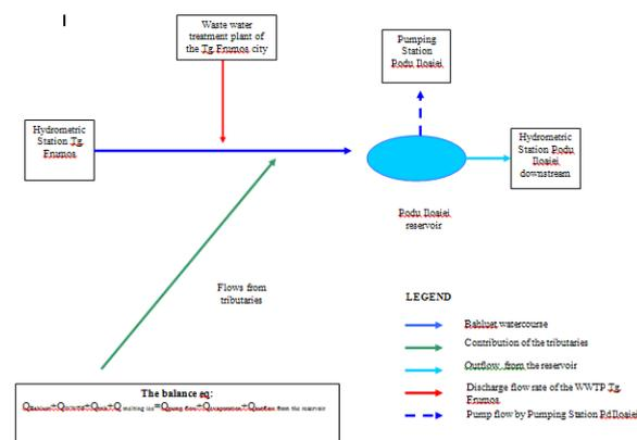
**Fig. 1-** Schematic diagram of the flows which are part of the balance eq.
