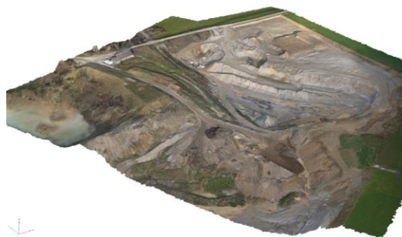
Fig. 4: 3D model obtained by automatic aerial photogrammetry
