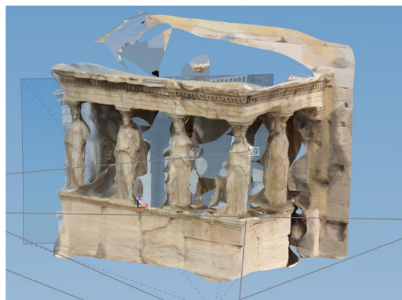
Fig. 2: 3D model obtained by automatic terrestrial photogrammetry
