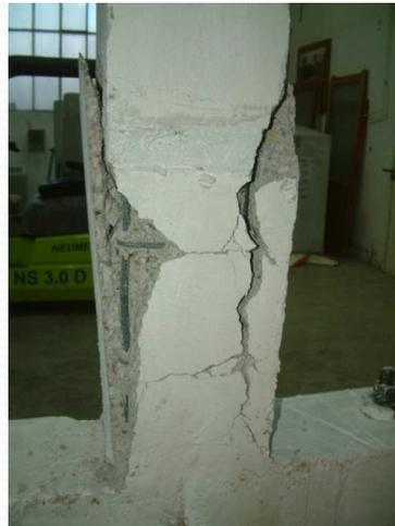
Figure 6.2 : Observed failure mechanism in experimental.
