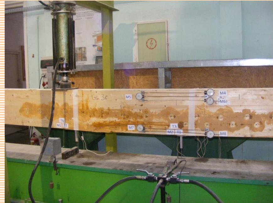
**CONSOLIDATION WITH FRP OF GLUED-LAMINATED TIMBER BEAMS**
