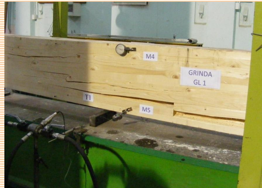
**CONSOLIDATION WITH FRP OF GLUED-LAMINATED TIMBER BEAMS**
