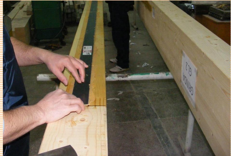
**CONSOLIDATION WITH FRP OF GLUED-LAMINATED TIMBER BEAMS**
