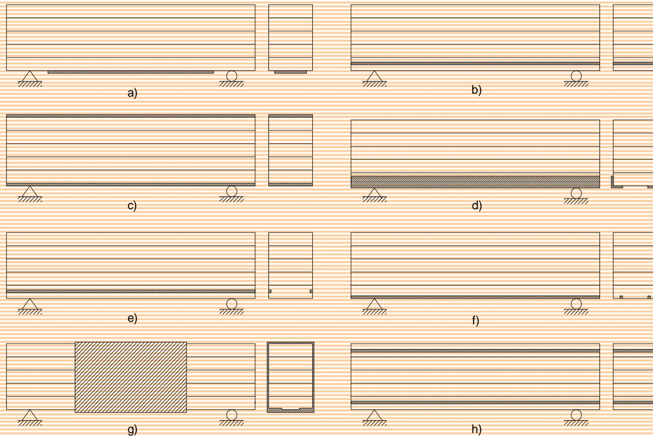
**CONSOLIDATION WITH FRP OF GLUED-LAMINATED TIMBER BEAMS**
