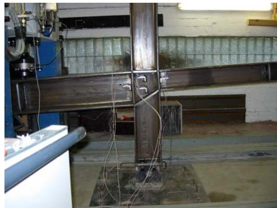
Figure 9b. Deformed shape before failure.
