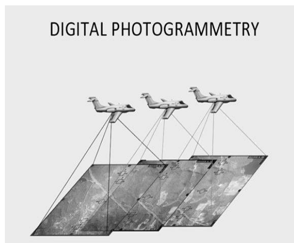
Figure 6. The principle of digital photogrammetry
