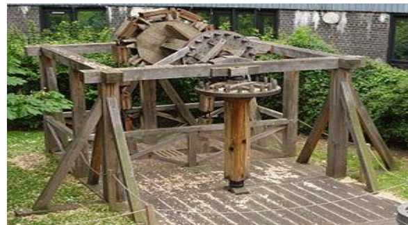
Figure 2. Reconstruction of a Roman pump
