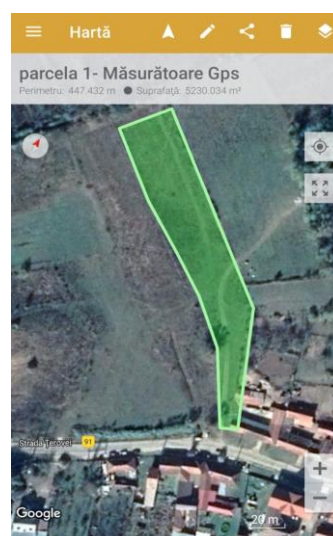
Figure 15. Measuring 39164 immovable's surface with GPS FieldsAreaMeasure mobile application using the command "GPSMeasurement"
