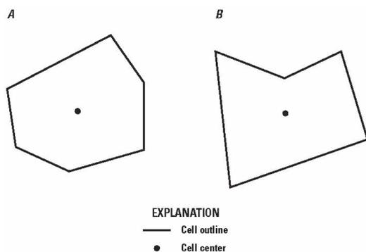
**Fig. 3.** Examples of A, convex and B, concave polygons. A convex polygon is one in which all interior angles are less than or equal to 180 degrees. A concave polygon has at least one interior angle that is greater than 180 degrees. MODFLOW-USG cells should have a convex shape.
