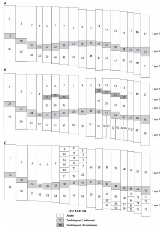
**Fig. 5.** Types of layering schemes that can be used with MODFLOW-USG: A, the grid configuration is the same for all layers; B, the grid configuration is different for different layers, and C, one or more layers contain vertical subdivision.
