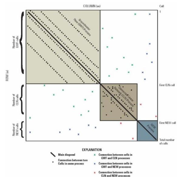
**Fig. 1.** Conductance matrix in MODFLOW-USG illustrating the framework for tightly coupling cells with cells from other processes.
