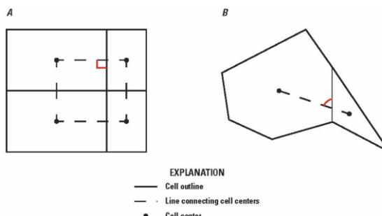
**Fig. 2.** Examples of two different types of cell connections: A, a line connecting the centers of adjacent cells passes through the shared face at a right angle, and B, a connecting line does not intersect the shared face at a right angle.
