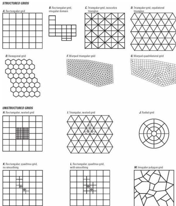
**Fig. 4.** Examples of different types of structured and unstructured grids.
